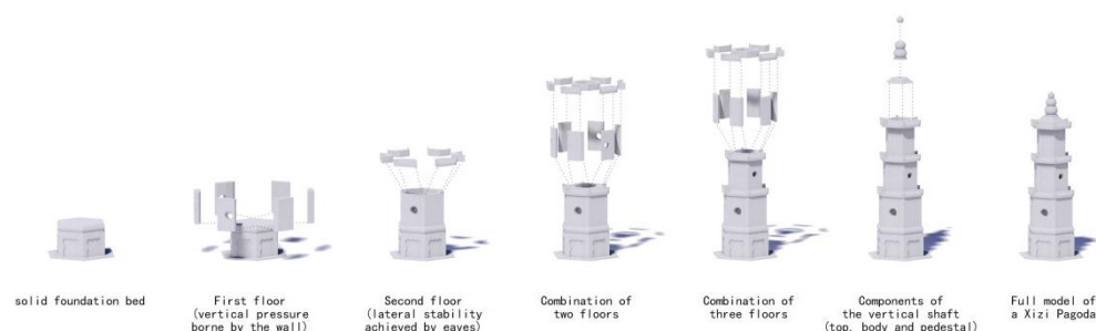
Figure 9. Construction steps of the Xizi Pagoda and components of the solid foundation bed (image source: made by the author).
