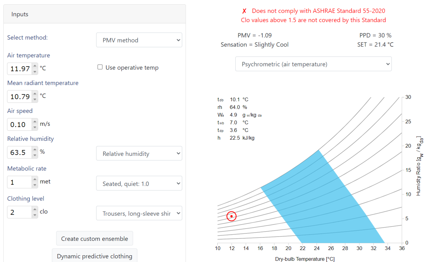
Figure 8. Psychrometric chart for the comfort condition (blue area) defined by Case ii input from Table 2 (red point). The abscissa is the dry-bulb temperature and the ordinate is the Humidity Ratio (HR%). The CBE comfort tools automatically calculates the relative air speed and the dynamic clothing insulation [49,52].
