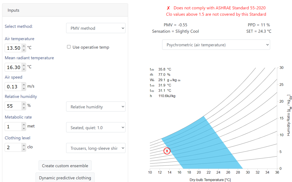
Figure 11. Psychrometric chart for the comfort condition (blue area) defined by Case ii input from Table 3 (infrared laps on: red point on the chart). The abscissa is the dry-bulb temperature and the ordinate is the Humidity Ratio (HR%). The CBE comfort tools automatically calculates the relative air speed and the dynamic clothing insulation [49,52].
