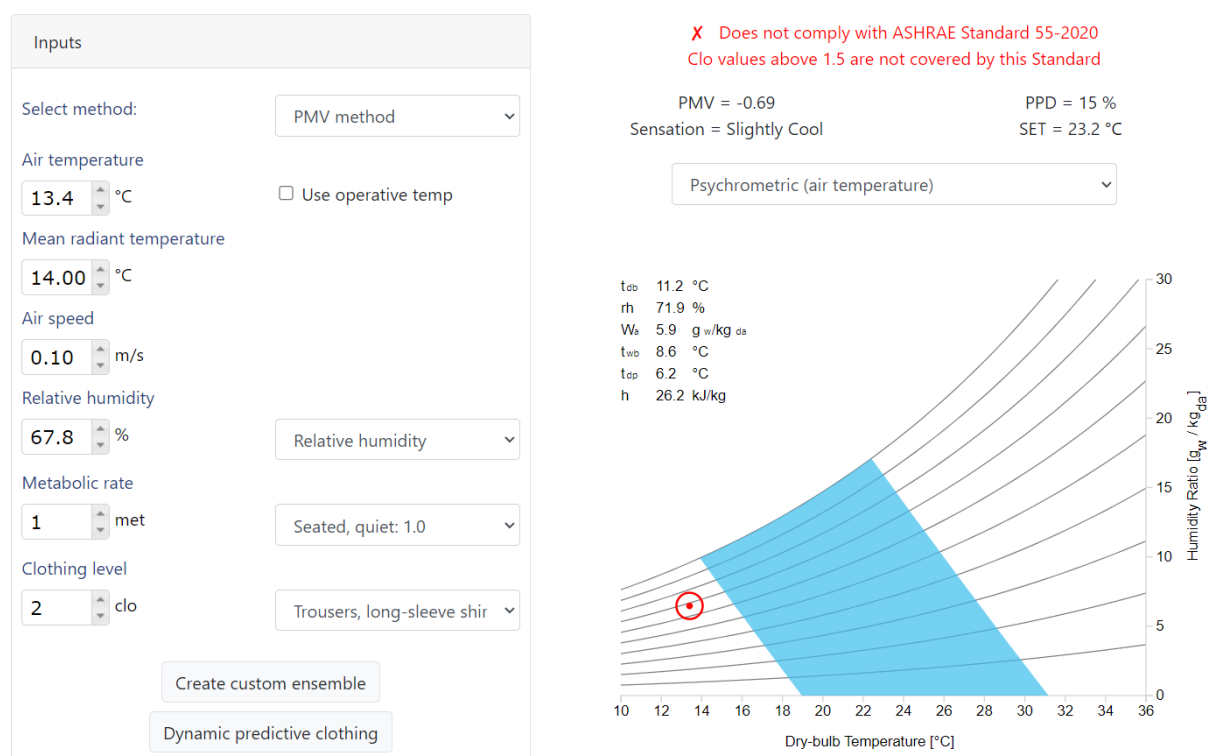
Figure 6. Psychrometric chart for the comfort condition (blue area) defined by Case ii input from Table 1 (red point). The abscissa is the dry-bulb temperature and the ordinate is the Humidity Ratio (HR%). The CBE comfort tools automatically calculates the relative air speed and the dynamic clothing insulation [49,52].
