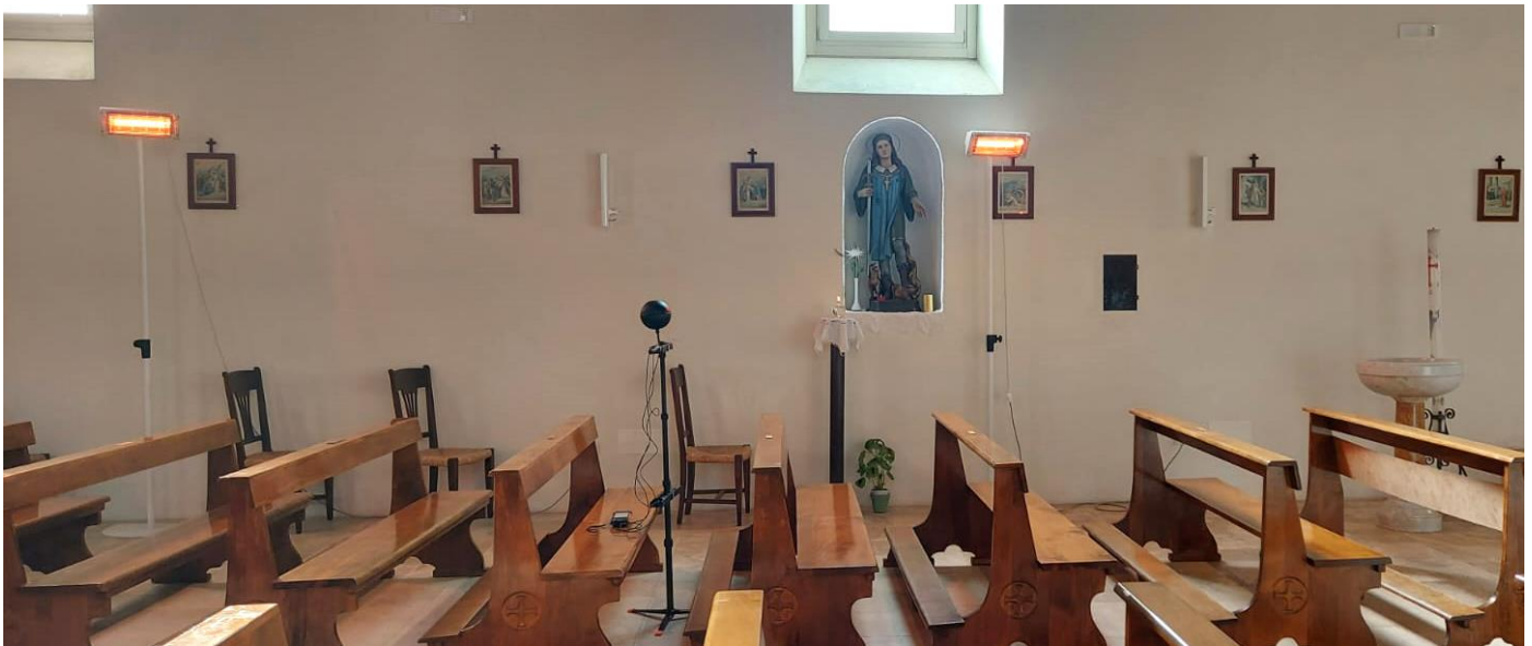
Figure 9. Comfort monitoring of the S. Vito church: Case ii and infrared lamps on.
