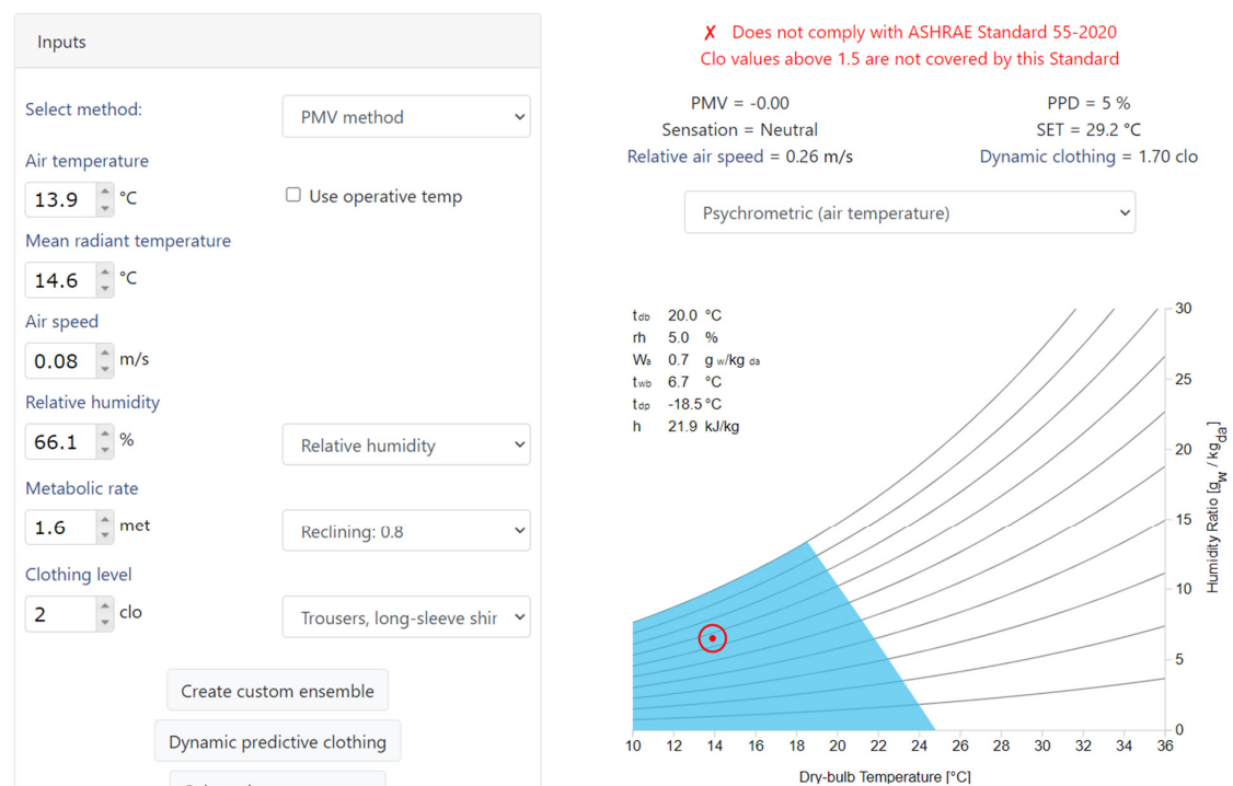
Figure 5. Psychrometric chart for the comfort condition (blue area) defined by Case i input from Table 1 (red point). The abscissa is the dry-bulb temperature and the ordinate is the Humidity Ratio (HR%). The CBE comfort tools automatically calculates the relative air speed and the dynamic clothing insulation [49,52].
