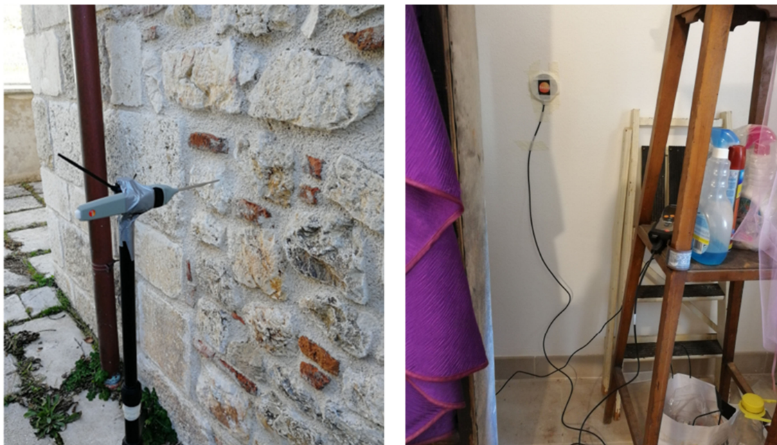
Figure 3. The heat-flow analysis carried out: the monitoring phase on the church masonry.
