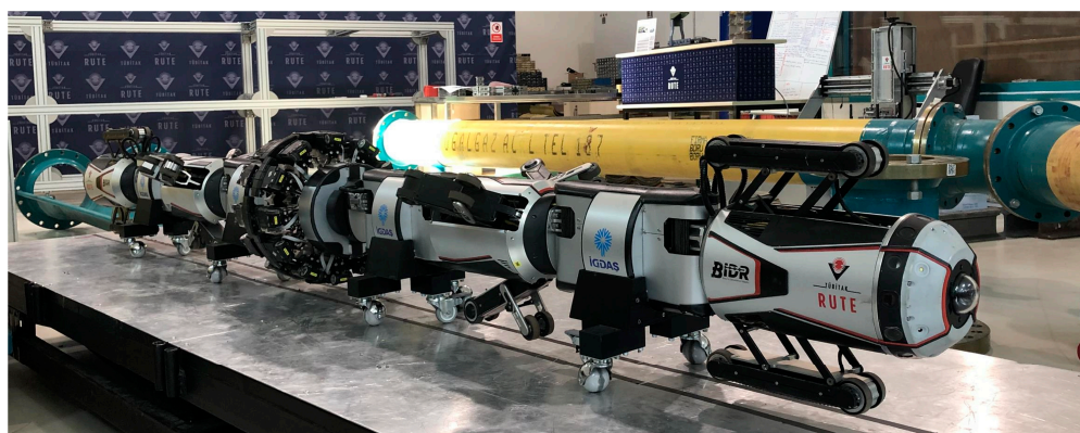
Figure 1. The natural gas inspection robot.
