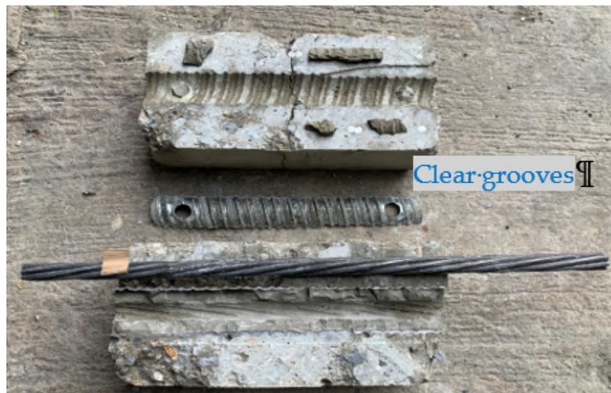
**Figure 13.** Bonding interface between strand and grout in Specimen I-60-270P1.
