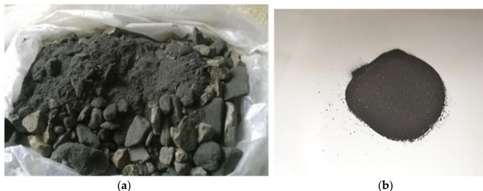
**Figure 2.** (a,b) The material from the top layer and homogenized, sieved material under 1 mm (source: elaborated by authors).
