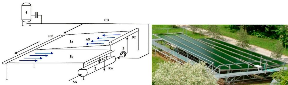
**Figure 1.** The phototrophic cultivation cascade—a schematic drawing and an overall photo [9,30]. legend: 1 a,b—cultivation areas; 2—a collection tank; 3—a circulation pump; 4—a carbon dioxide reservoir; AA—algae suspension generation; AS—algae suspension flow; CC—a connecting trough; CD—a distribution pipe; DT—a transition trough; Rw—rainwater and washing water.
