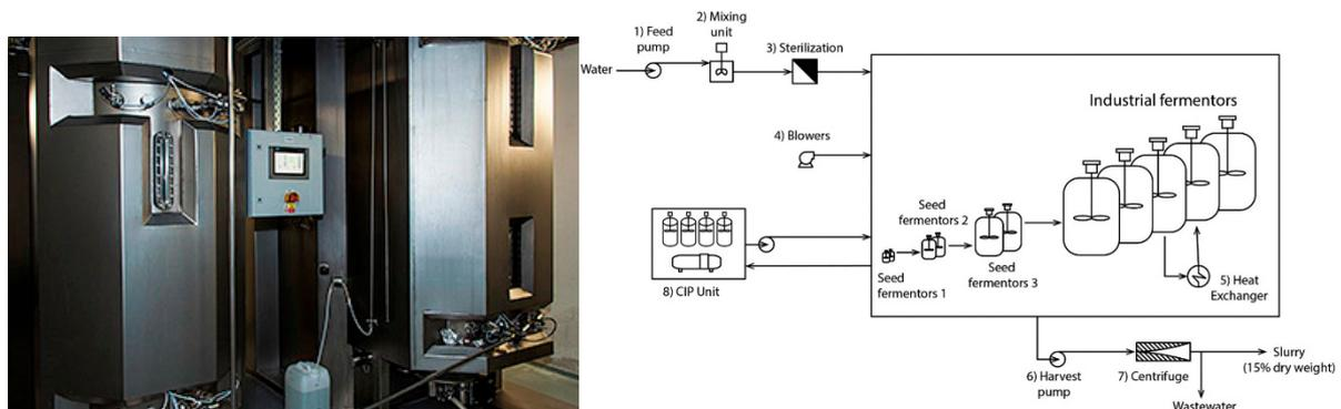
**Figure 2.** The heterotrophic fermenter—an overall photo and a typical scheme of the heterotrophic production [31,33]. Notes: CIP—cleaning in place.
