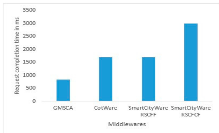
Figure 12. Comparison of GMSCA request completion time with other middleware.
