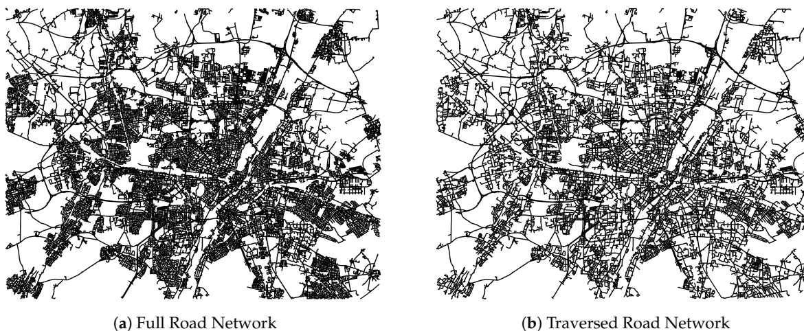
Figure 4. Comparison between the (a) full road network for Munich, Germany, and the (b) network composed of edges that have been traversed at least once during Random Route Sampling.
