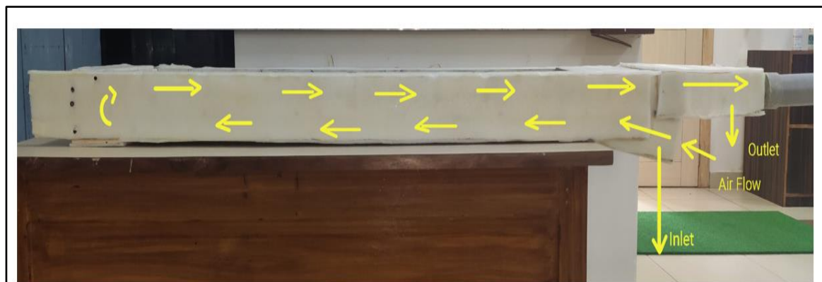
Figure 3. Direction of flow of air inside the duct.
