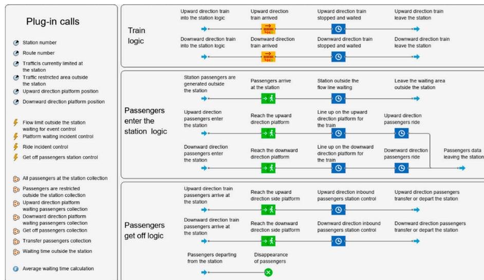
Figure 6. Passengers, train logic, and main plug-in calls in the station agent.
