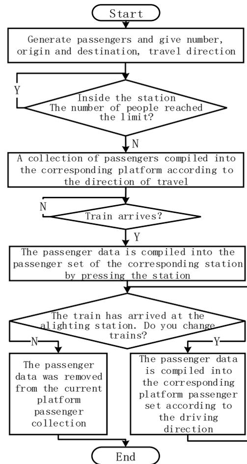
**Figure 4.** Logic flow chart of single passenger data processing.
