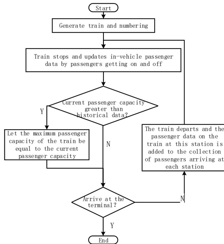
**Figure 5.** Logic flow chart of data processing for a single train agent.
