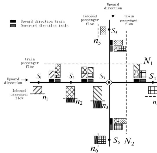
**Figure 1.** Schematic diagram of the passenger flow limiting of a two-line cross urban rail transit network.
