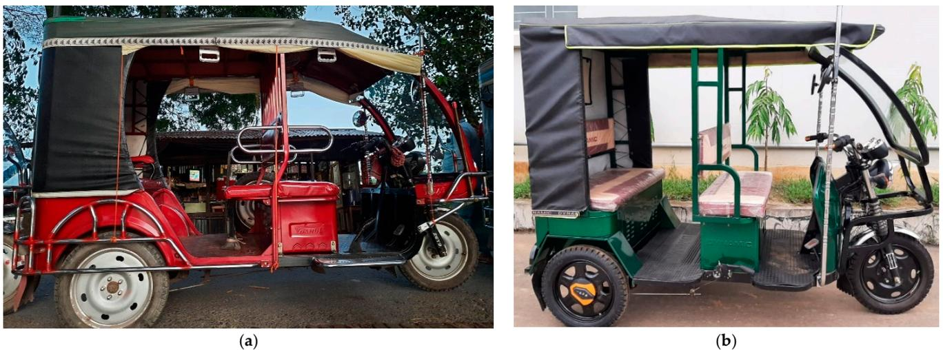
**Figure 1.** Electric three-wheelers: (a) Easy Bike (b) Mishuk.
