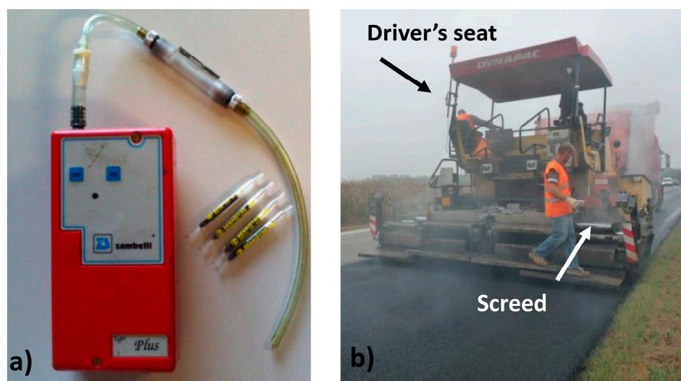
**Figure 1.** (a) Pump and cartridges used to collect the asphalt fumes, (b) positions where the fumes were collected at the paver.
