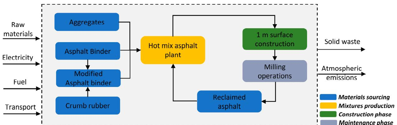
**Figure 2.** System boundaries for 1 m of the road wearing course construction.
