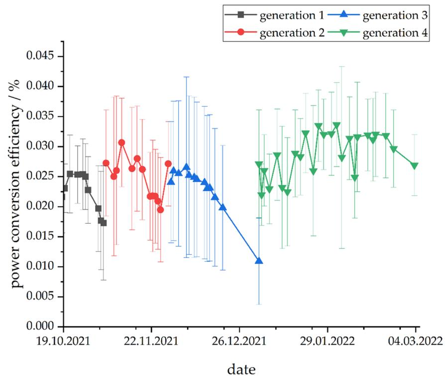
**Figure 2.** Average PCE of four generations of DSSCs with commercially applied TiO<sub>2</sub> layers.
