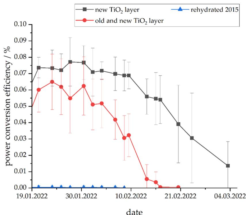
**Figure 7.** Average PCE of 18 DSSCs from 2015 with manually applied TiO<sub>2</sub> layers. The grey line is the DSSCs with a new TiO<sub>2</sub> layer on cleaned glass, the red line is the DSSCs with new TiO<sub>2</sub> layers on top of the old TiO<sub>2</sub> layer and the blue line is the DSSCs that were rehydrated with electrolyte.
