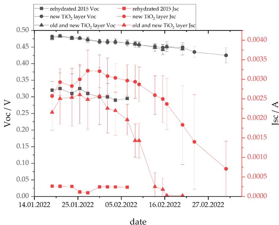
**Figure 8.** Average Voc and Jsc of 18 DSSCs from 2015 with manually applied TiO<sub>2</sub> layers. The round marks symbolize DSSCs with a new TiO<sub>2</sub> layer on cleaned glass, the triangle marks symbolize DSSCs with new TiO<sub>2</sub> layers on top of the old TiO<sub>2</sub> layer and the square marks symbolize DSSCs that were rehydrated with electrolyte.
