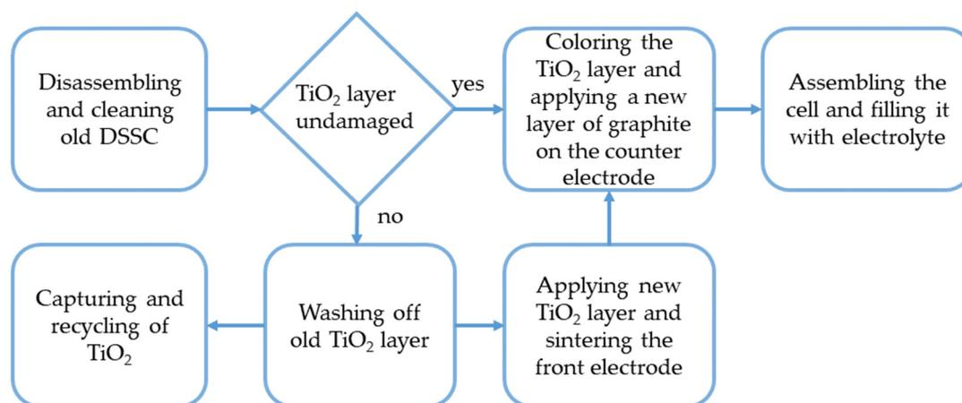
**Figure 1.** Visualized process of remanufacturing DSSCs.
