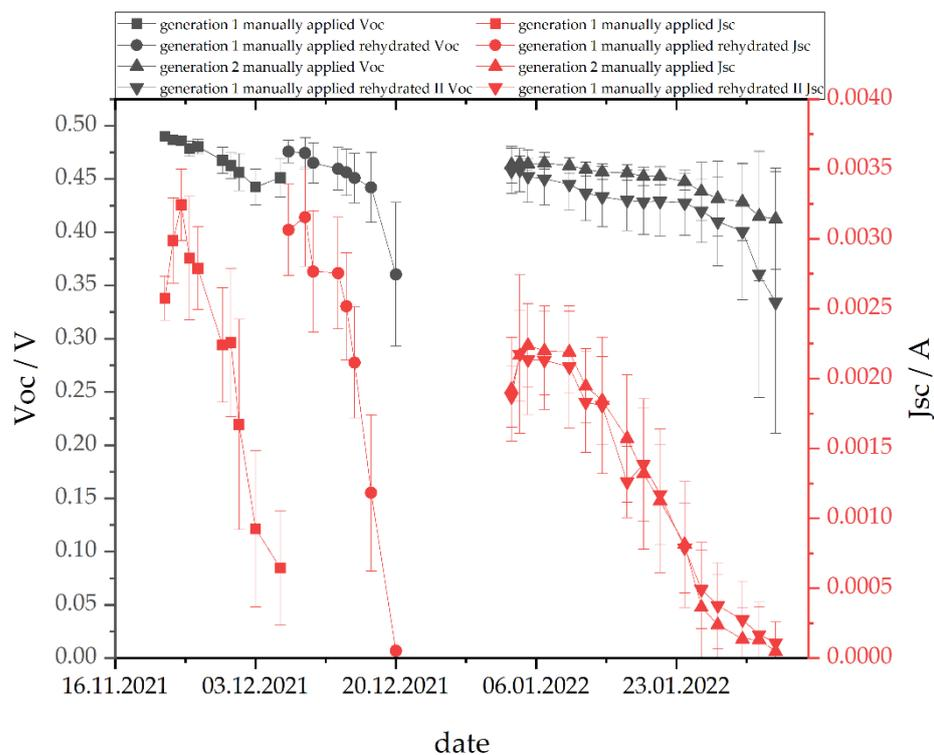
**Figure 6.** Average Voc and Jsc of 12 DSSCs with manually applied TiO<sub>2</sub> layers. The third generation was split into six DSSCs that were remanufactured and six DSSCs that were refilled with electrolyte.
