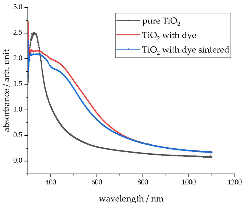
**Figure 10.** UV-Vis absorption spectra of pure TiO<sub>2</sub>, TiO<sub>2</sub> with dye from a used DSSC and a used TiO<sub>2</sub> layer after sintering in the oven.
