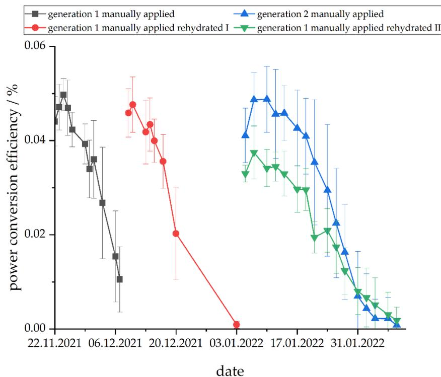
**Figure 5.** Average PCE of 12 DSSCs with manually applied TiO<sub>2</sub> layers. The third generation was split into six DSSCs that were remanufactured and six DSSCs that were refilled with electrolyte.
