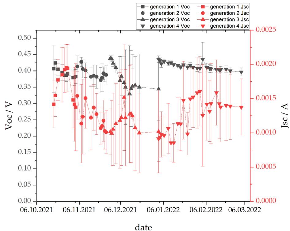
**Figure 3.** Average Voc and Jsc of four generations of DSSCs with commercially applied TiO<sub>2</sub> layers.
