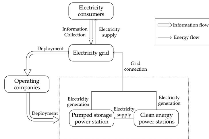
**Figure 2.** Combined operation mode of wind power and pumped storage.
