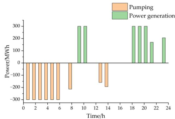
**Figure 4.** Pumping strategy of pumped storage power station.
