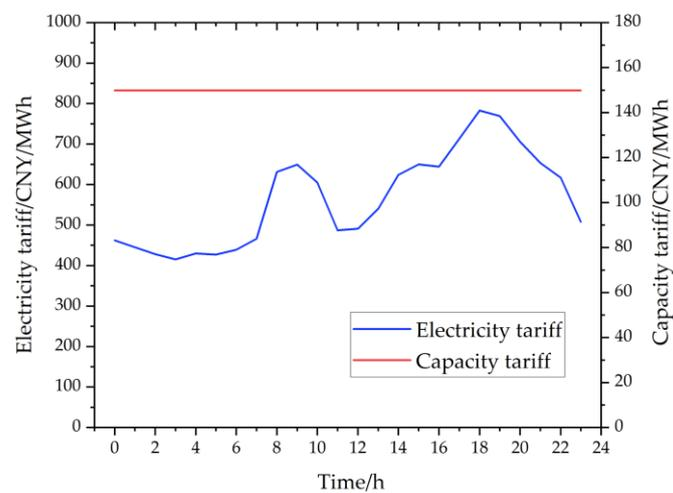
**Figure 5.** Two-part tariff for pumped storage.
