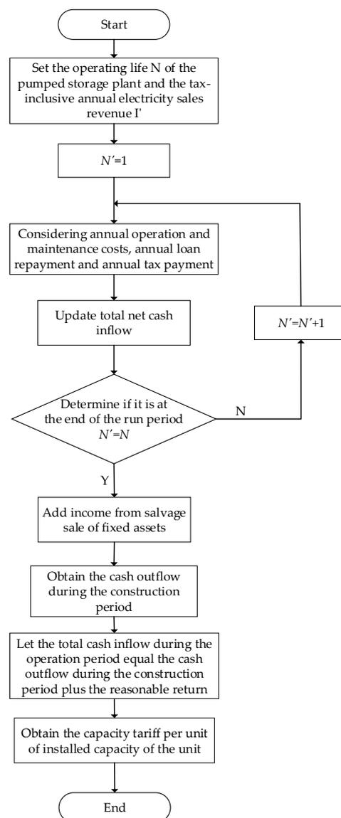
**Figure 1.** Flow chart of capacity tariff solving.
