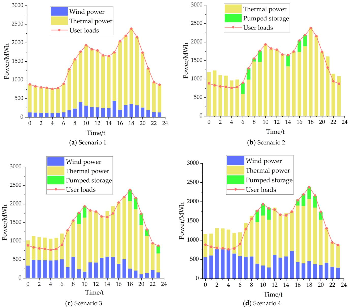
**Figure 6.** Output of different units in four scenarios.
