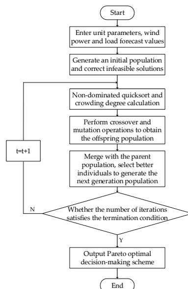
Figure 3. Flow chart of electricity price solution.
