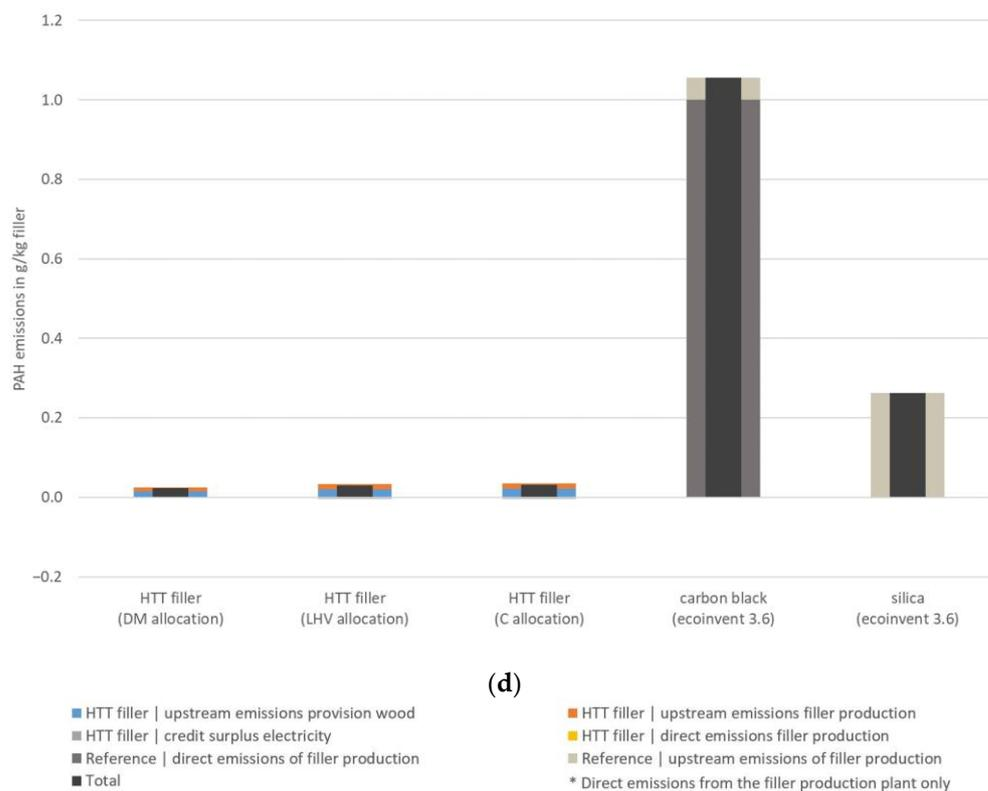
**Figure 5.** Cradle-to-gate SO<sub>2</sub> emissions (a), NO<sub>x</sub> emissions (b), PM emissions (c) and PAH emissions (d) of the HTT filler and of the reference fillers carbon black and silica. DM = dry matter; LHV = lower heating value; C = carbon.
