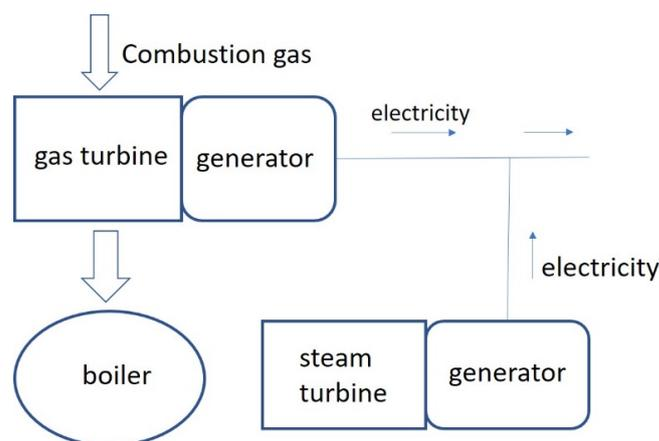
**Figure 2.** Basic NG combined cycle power generation.
