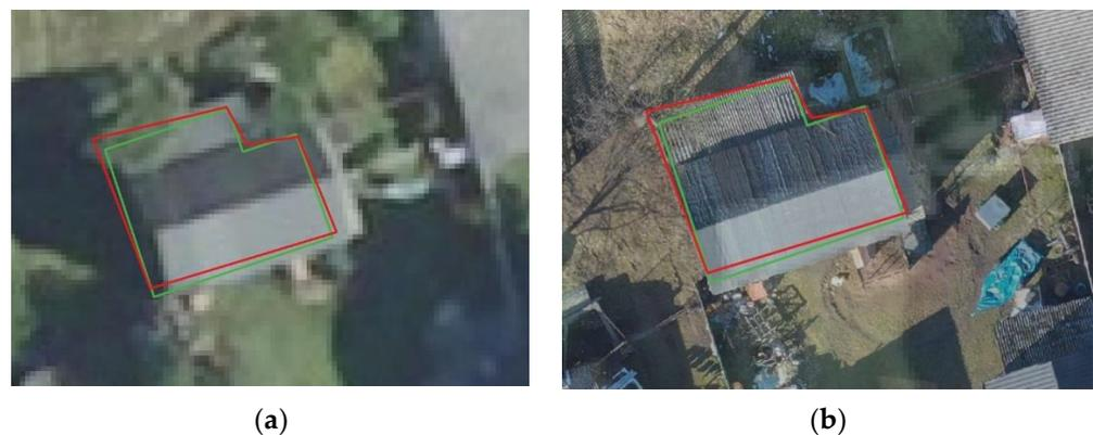
**Figure 10.** The results of measurements on the basis of the GNSS RTK method (green) and a photogrammetric forward section (red) against a background of an orthophoto map from the national geoportal (a) and prepared on the basis of UAV images (b).
