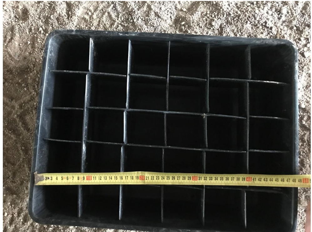
Figure 2. Top view of experimental test boxes used to determine the transverse irregularities of fertilizer application.
