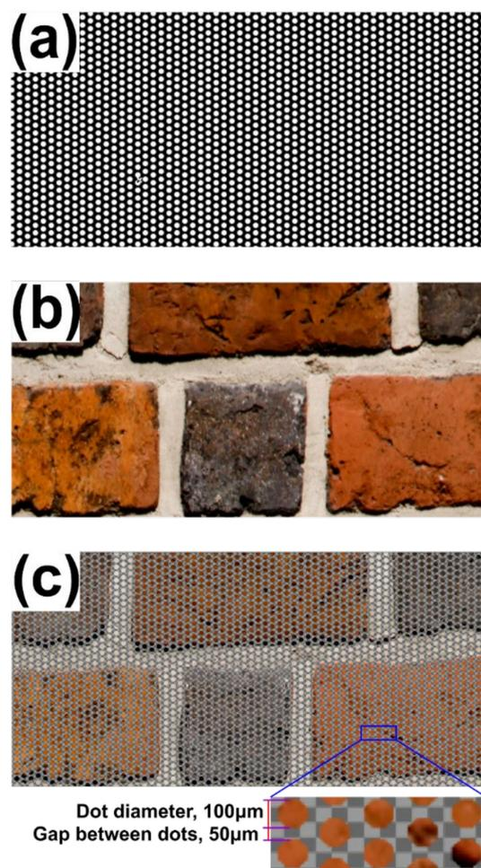
**Figure 2.** Generation of micropatterned image: (a) micropattern produced by Python, (b) high-resolution wall image, and (c) micropatterned image where the dot diameter is 100 μm, and the gap between the dots is 50 μm.
