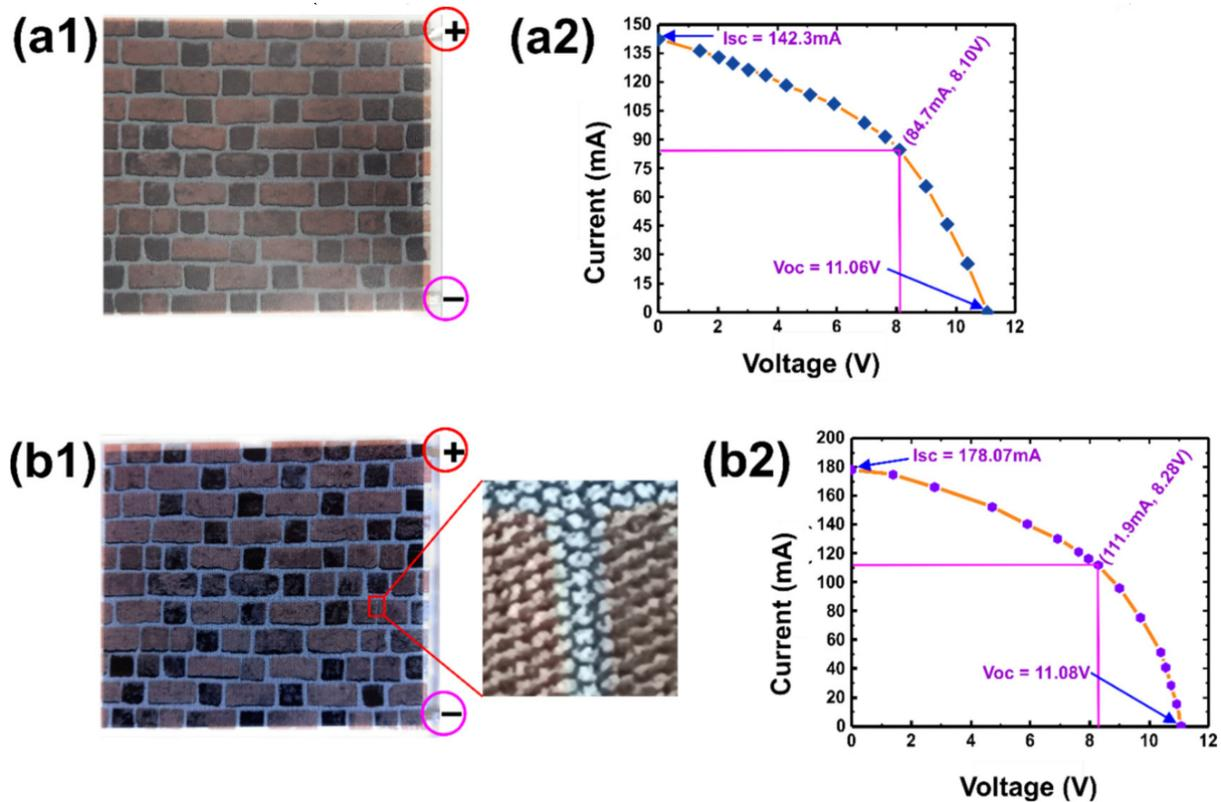
**Figure 5.** Multicolored brick-look PV module (a1) and its I-V characteristics diagram (a2) and micropatterned-based colored PV module (b1) and its I-V curve (b2).
