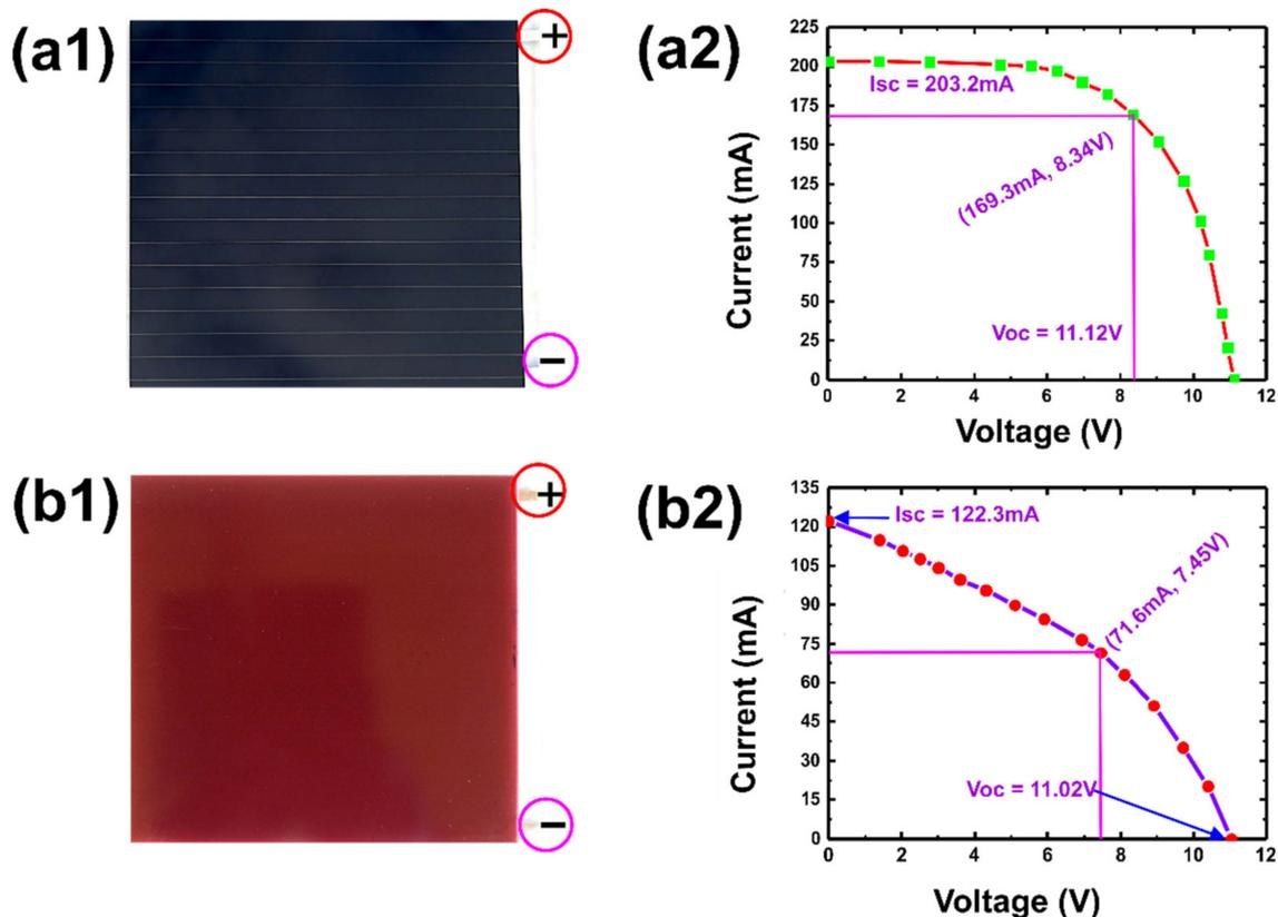
**Figure 4.** Physical appearance (a1) and its I-V characteristics diagram (a2) of the standard PV module and visual appearance (b1) and its I-V curve (b2) of single-colored PV modules.
