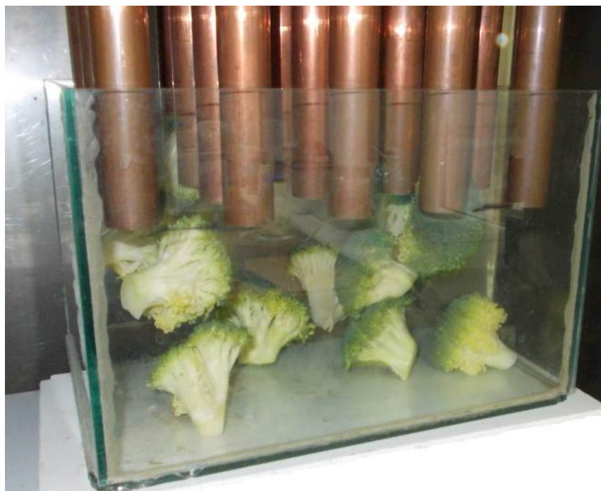
Figure 9. Boiling bed of a single layer of broccoli rosettes subjected to the impingement fluidization treatment.
