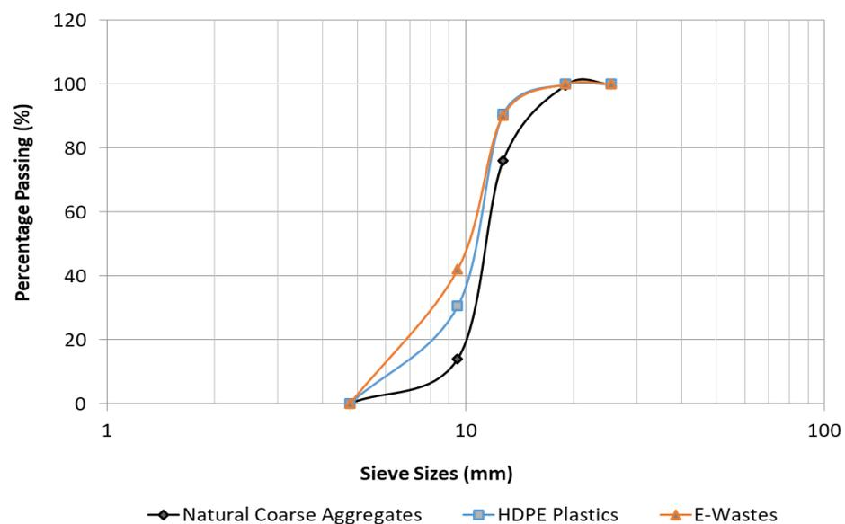
**Figure 3.** Particle size distribution curve for natural and plastic aggregates.
