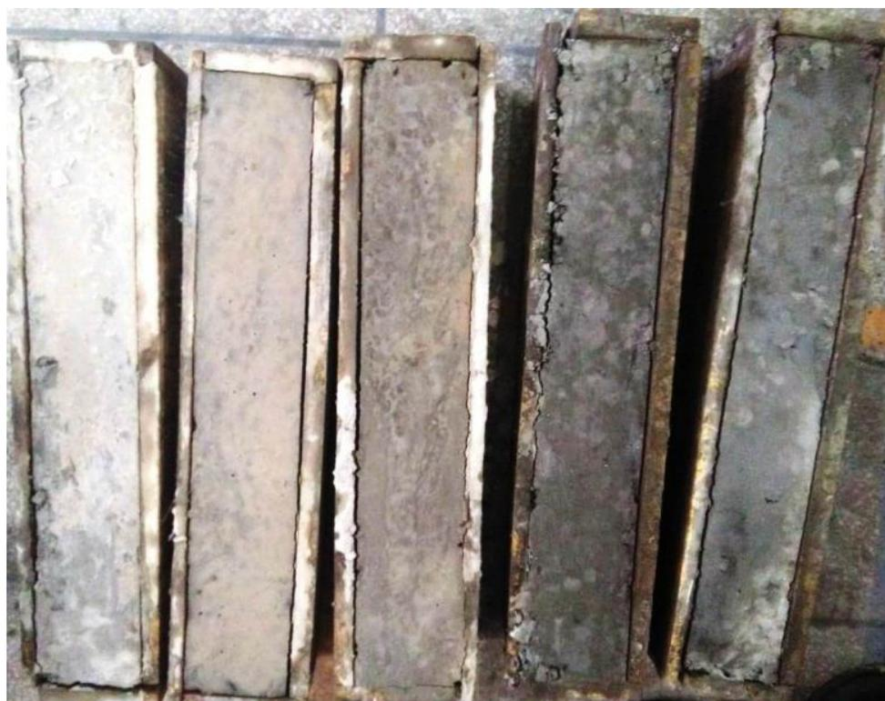
**Figure 16.** Simple concrete beams for flexural strength test.
