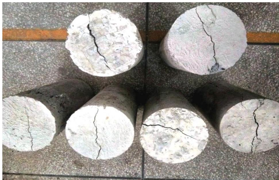
**Figure 13.** Failure mode of concrete cylinders with recycled plastics after split tensile strength test.
