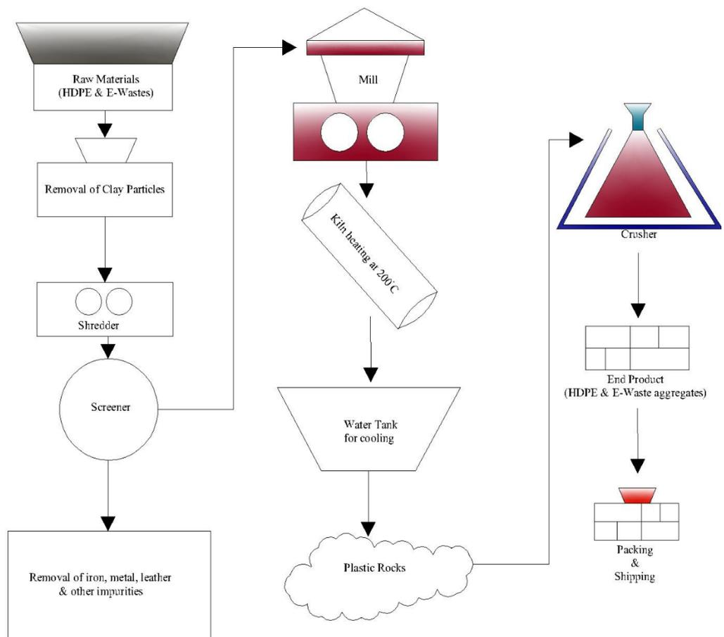
**Figure 5.** Schematic diagram of the manufacturing process of HDPE and E-wastes.
