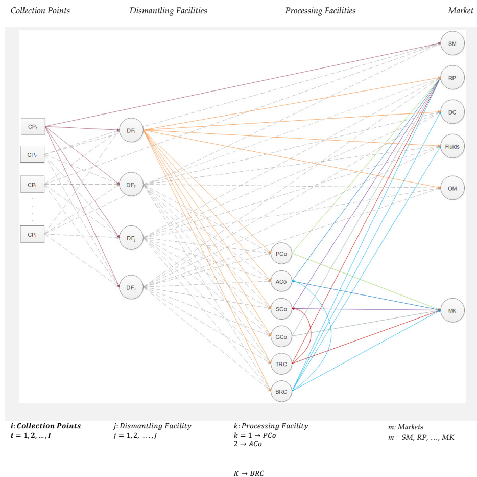
Figure 2. Proposed Network: burgundy, ELVs flow; orange, parts flow; green, plastics flow; dark blue, aluminum flow; purple, steel flow; solid gray, glass flow; red, tire flow; blue, battery flow; dashed gray, future interactions/flows.
