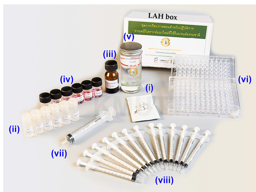
Figure 1. LAH box set: (i) a sachet of Nat Pow Iron, (ii) vials containing Fe(III) standard and sample solutions, (iii) a bottle of acetic/acetate buffer solution, (iv) vials containing dye solutions, (v) a natural reagent extracting bottle, (vi) a 96-well plate, (vii) a 10-mL disposable syringe, and (viii) 1-mL disposable syringes.
