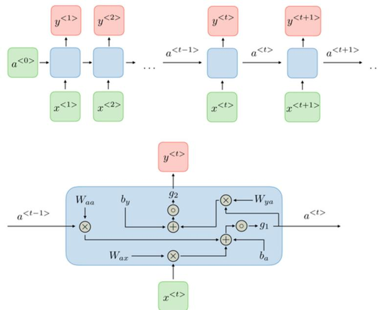
**Figure 1.** A typical schematic for recurrent neural networks (RNNs).
