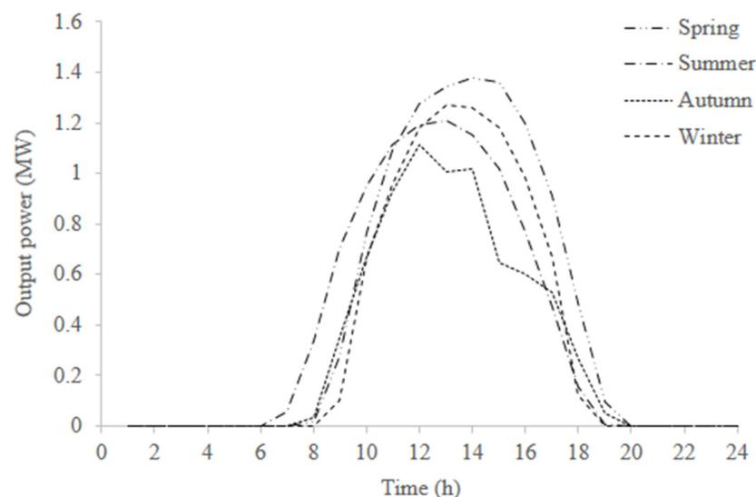
**Figure 2.** Variation in output power of the system versus time.
