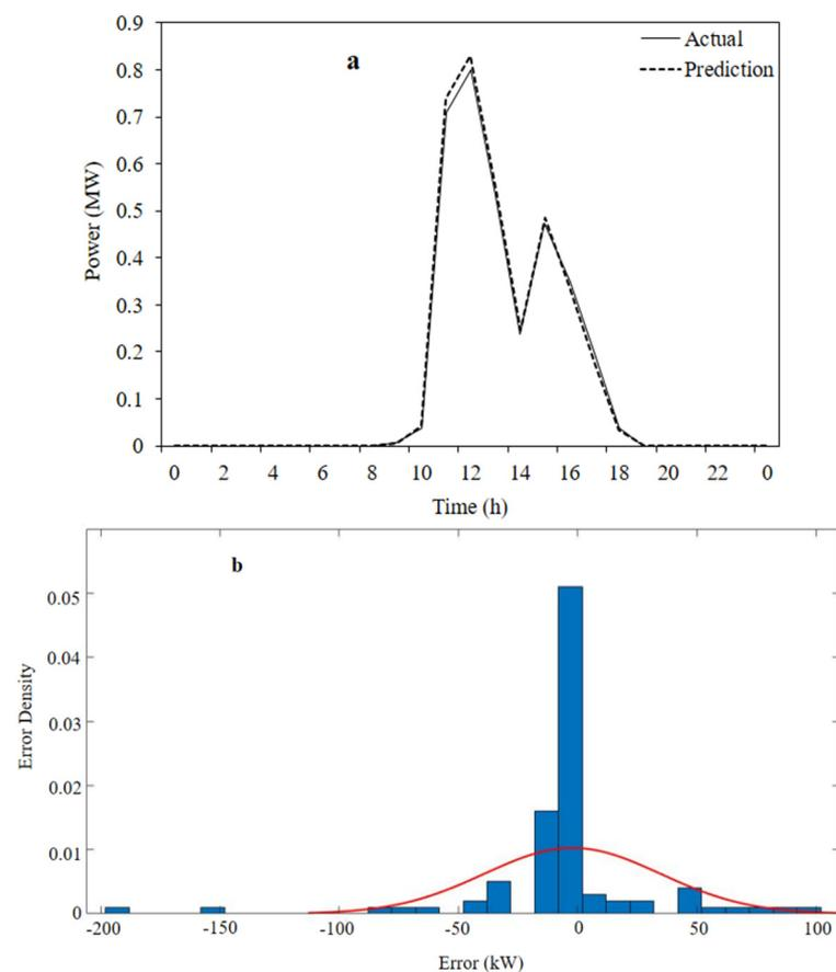
**Figure 7.** Prediction of power output of the PVPS on 25 December 2019 (a) and histogram and normal distribution of error (b).
