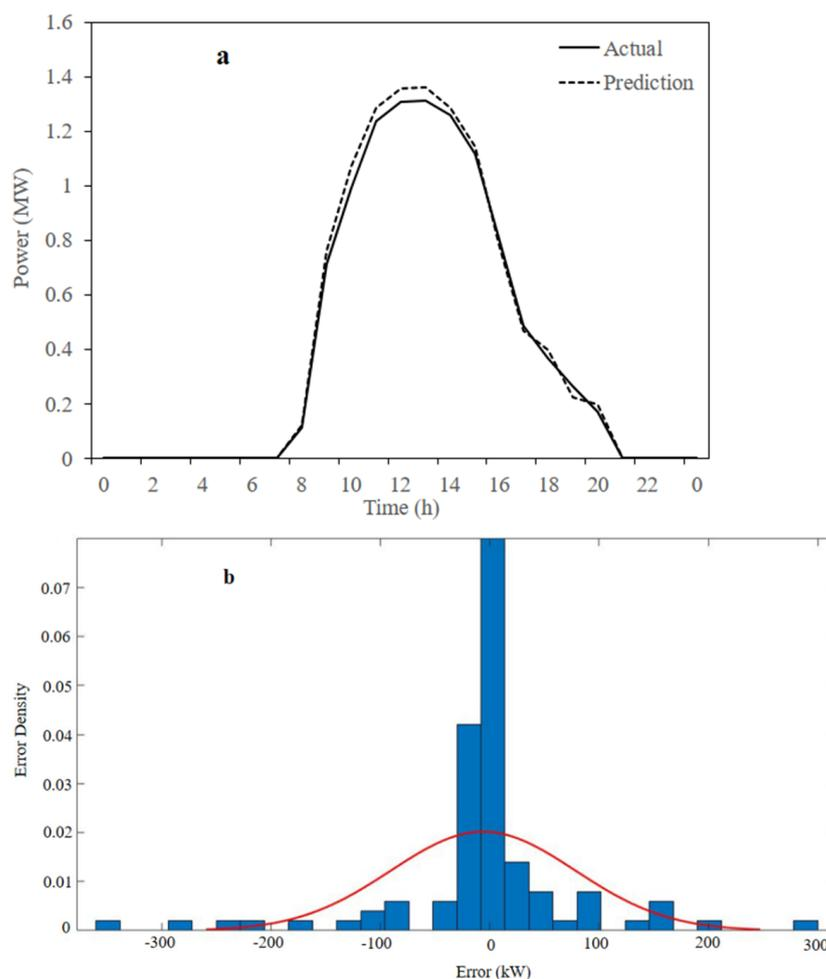
**Figure 8.** Prediction of power output of the PVPS on 25 December 2019 (a) and histogram and normal distribution of error (b).
