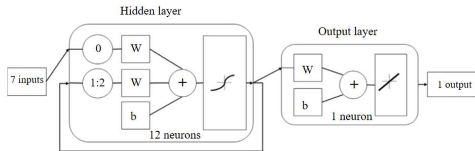
**Figure 3.** Diagram of the optimally designed RNN to model solar energy generation.
