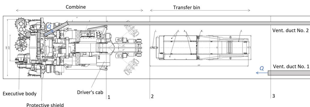
**Figure 1.** The position of the combine, transfer bin, and ventilation ducts in the dead-end drift (top view); measuring Sections 1, 2, and 3.
