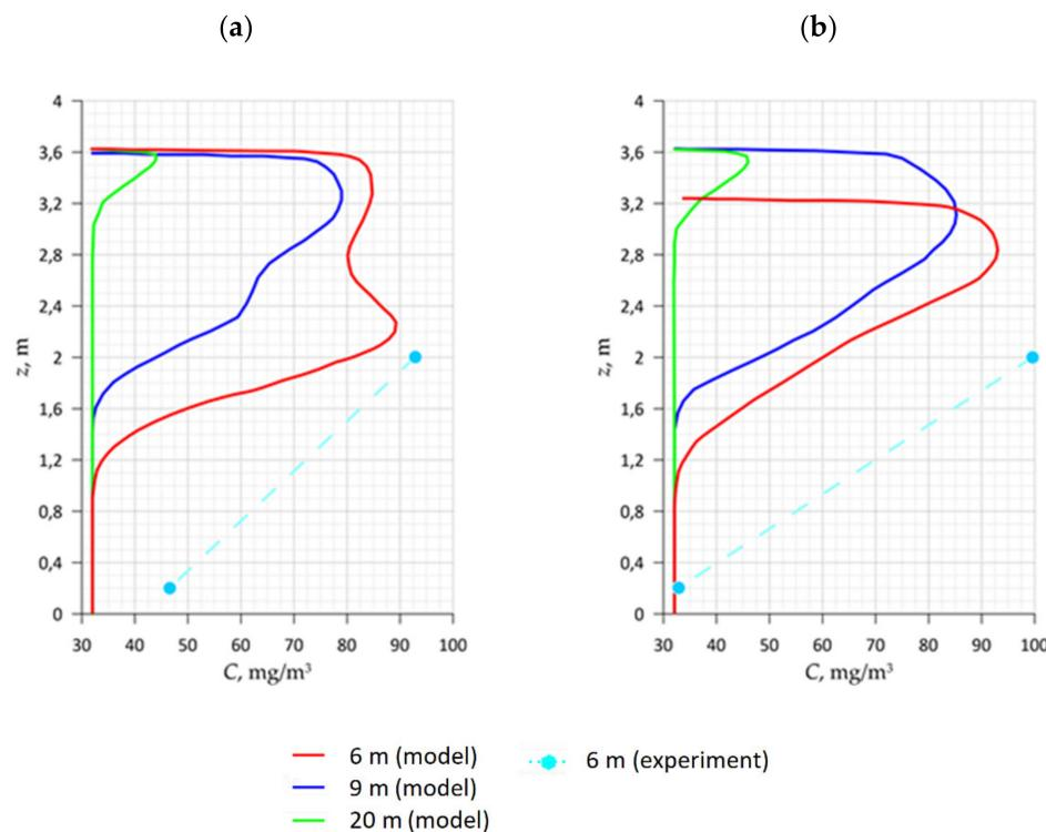
**Figure 5.** Comparative analysis of the distribution of dimensional dust concentration along the vertical lines of Section 2 to the right (a) and to the left (b) of the combine, exhaust ventilation system.
