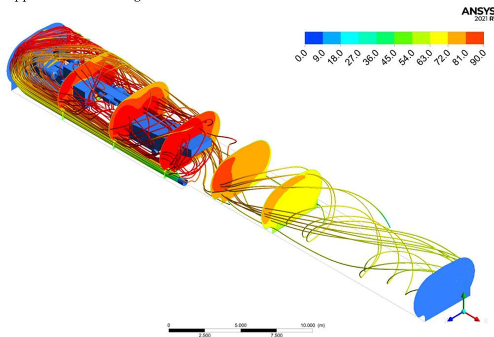
**Figure 7.** Calculated streamlines in a drift with forced ventilation system ( $Q = 3.8 \text{ m}^3/\text{s}$ ). The color shows the concentration of dust in the domain.
