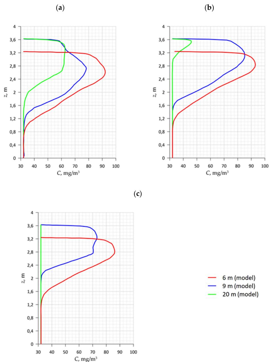
**Figure 9.** Mass concentration of dust at the measuring point near the combine for different air flow rates: (a)  $2.08 \text{ m}^3/\text{s}$ , (b)  $3.12 \text{ m}^3/\text{s}$ , (c)  $4.68 \text{ m}^3/\text{s}$ , exhaust ventilation system.
