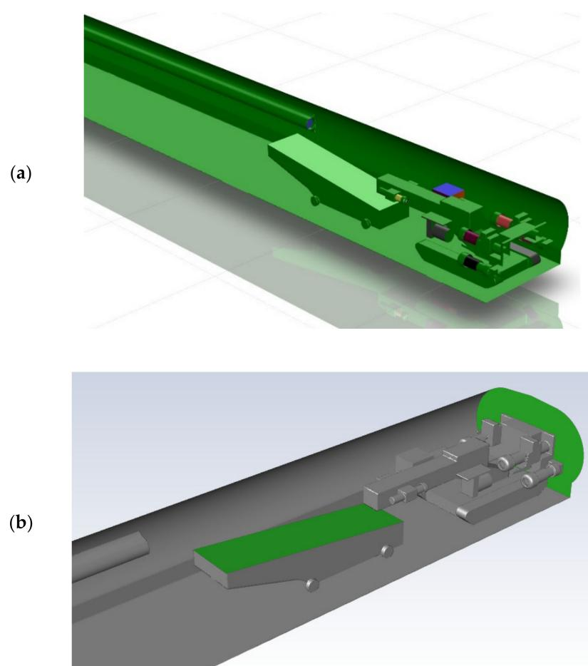
**Figure 3.** The geometry of the computational domain: (a) The combine engines (cylinders) and the driver's cab (rectangular block) are highlighted in color. (b) The surfaces where dust is generated are highlighted in color.
