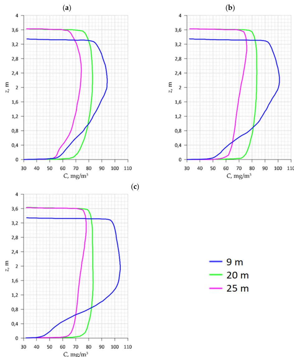
**Figure 8.** Dimensional dust concentration at the measuring point near the combine for different air flow rates: (a)  $1.9 \text{ m}^3/\text{s}$ , (b)  $3.8 \text{ m}^3/\text{s}$ , (c)  $7.6 \text{ m}^3/\text{s}$ , forced ventilation system.
