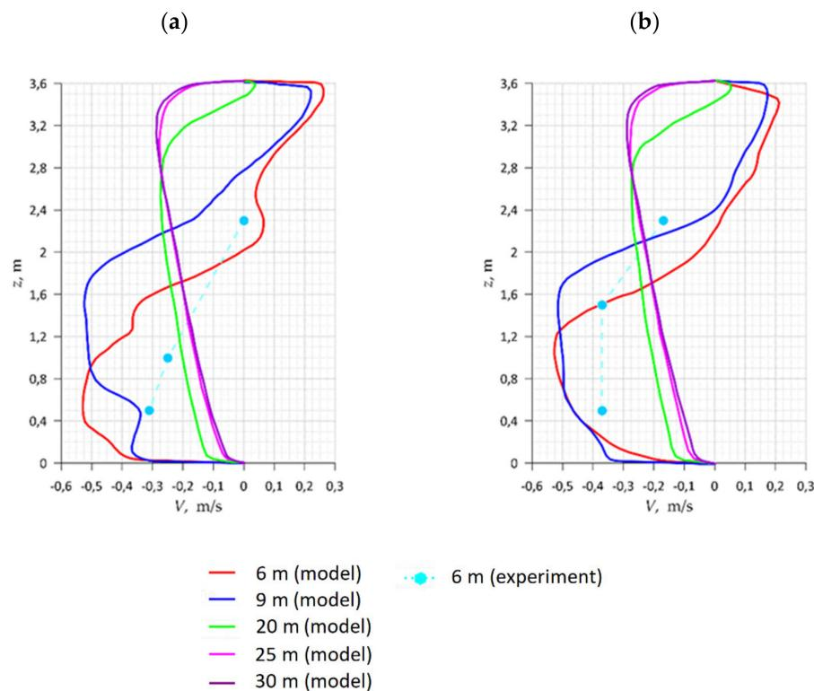
**Figure 6.** Comparative analysis of the distribution of the air flow velocity along the vertical lines of Section 2 to the right (a) and to the left (b) of the combine, exhaust ventilation system.
