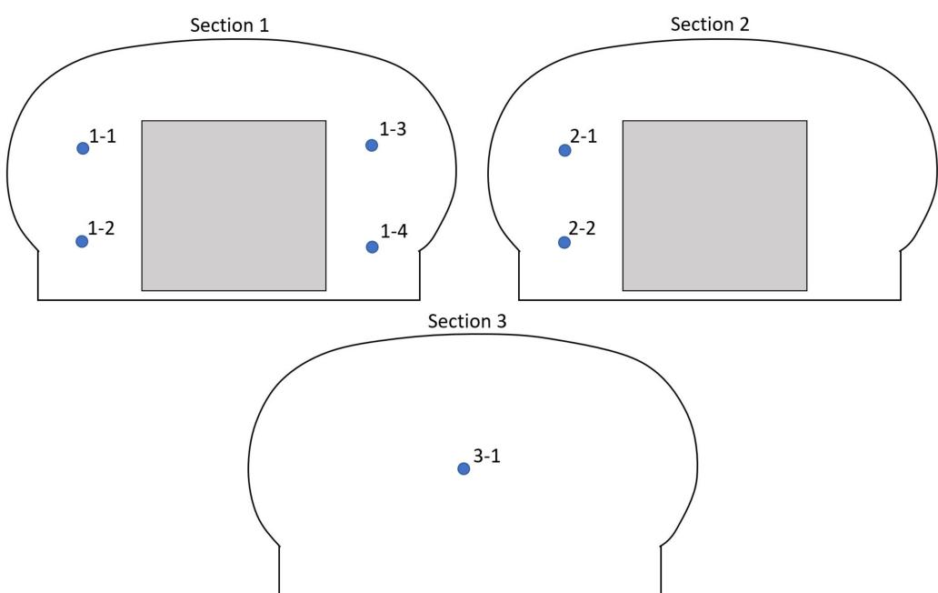
**Figure 2.** Dust measurement points for Sections 1, 2, and 3.
