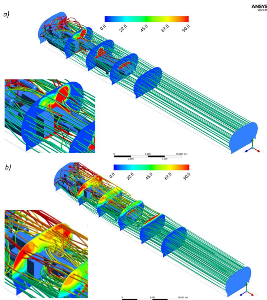
**Figure 10.** Dust–air mixture streamlines for exhaust ventilation at different intake fan positions: (a) 0.5 m from the protective shield, (b) opposite the combine driver's cab. The color shows the dimensional concentration of dust.
