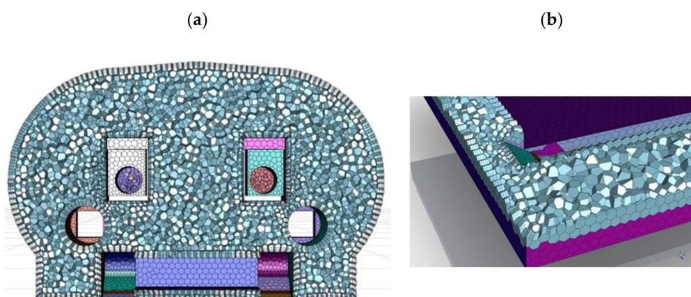
**Figure 4.** Computational mesh at (a) vertical cross-section of the combine and (b) near the mine wall.
