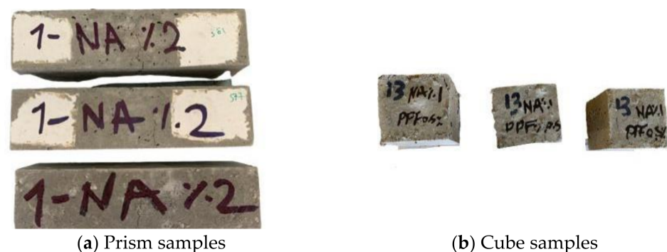
Figure 2. The cubic and prism specimens.
