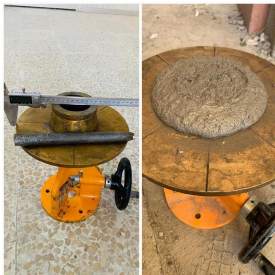
Figure 3. The flow table test.
