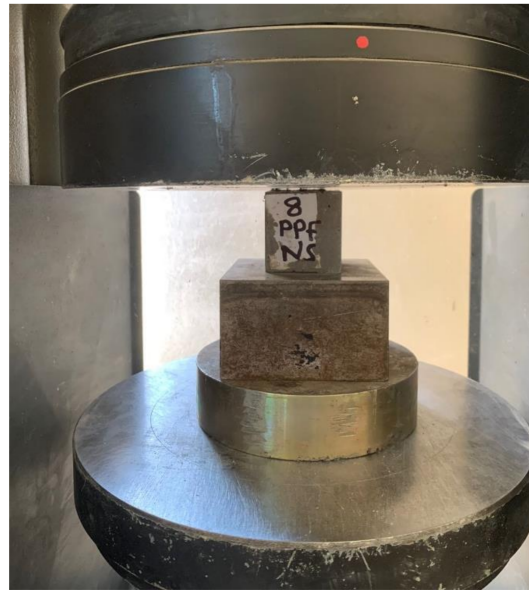
Figure 5. The compressive strength test of the alkali-activated mortar.
