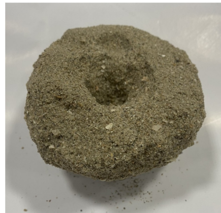
Figure 9. The consolidated column of the two-phase surface spray with injection (Case2-SI) treatment strategy.
