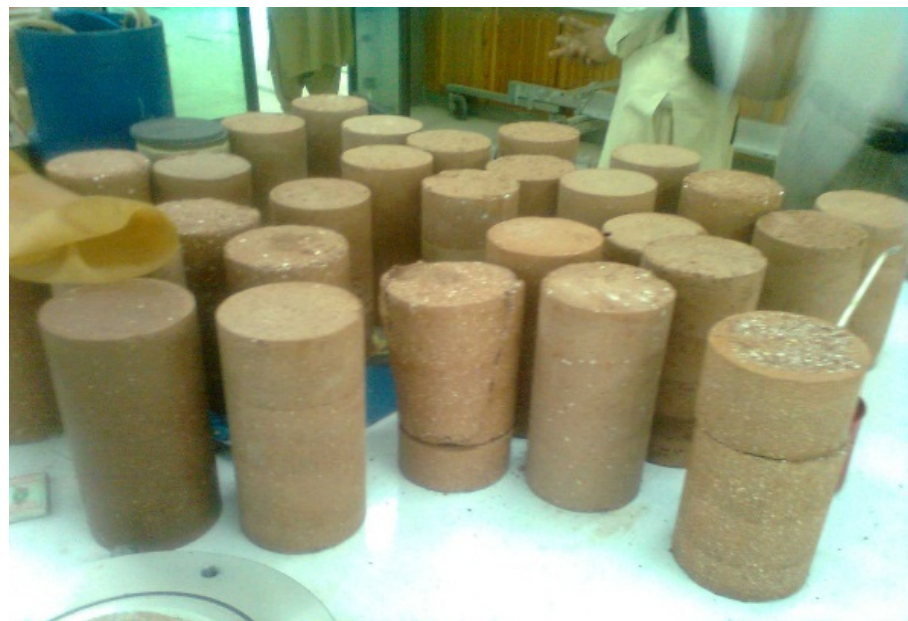
Figure 3. Specimens tested for resilient modulus test.
