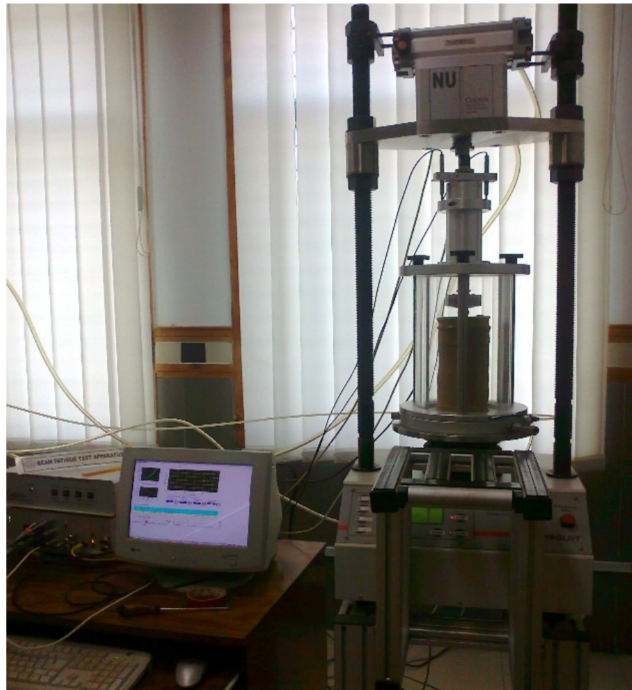
Figure 2. Setup of Triaxial test NU-14.
