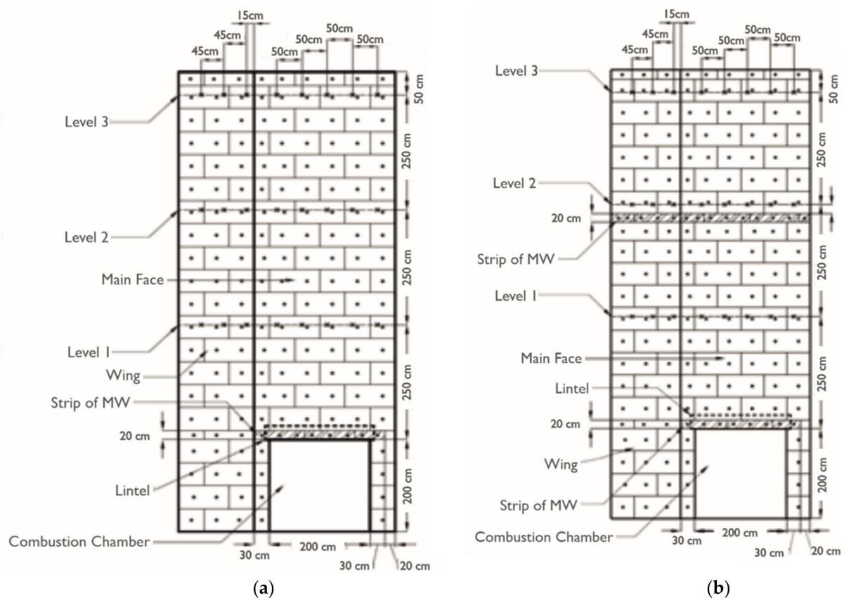
**Figure 3.** Scheme of the test wall: (a) insulation made of EPS with a 20 cm strip of MW placed in the overhead of the combustion chamber—variant III; (b) insulation made of EPS with a 20 cm strip of MW placed in the lintel of the combustion chamber and a 20 cm inter-story strip of MW located 5 m above the combustion chamber—variant IV.
