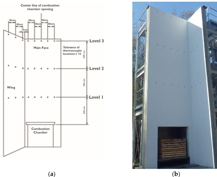
**Figure 1.** Test wall according to BS 8414-1: 2020 [10] (a) diagram showing the arrangement of measurement elements [10]; (b) removal of the wall before the test with a visible combustion chamber filled with a properly prepared pile of wood.
