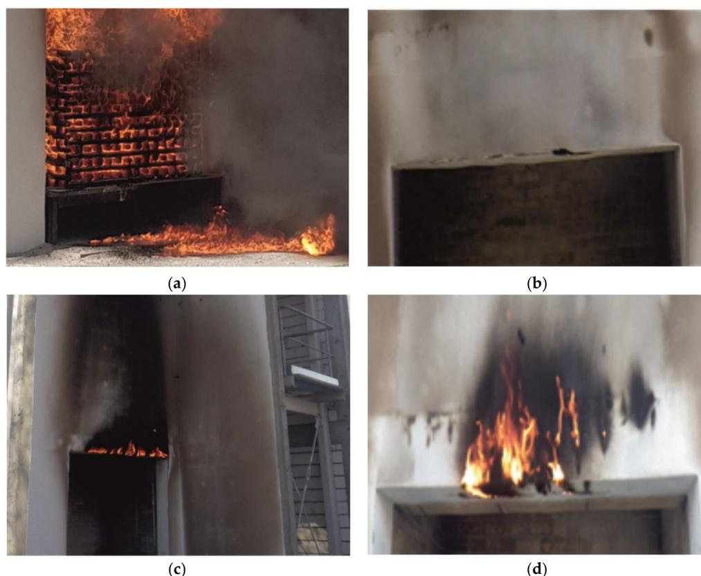
**Figure 4.** (a) View of the melted polystyrene in front of the combustion chamber—variant I; (b) view of the cracked EPS lintel—variant II; (c) view of the burning mineral wool lintel after completion of the test—variant III; (d) view of the burning mineral wool lintel after completion of the test—variant IV.
