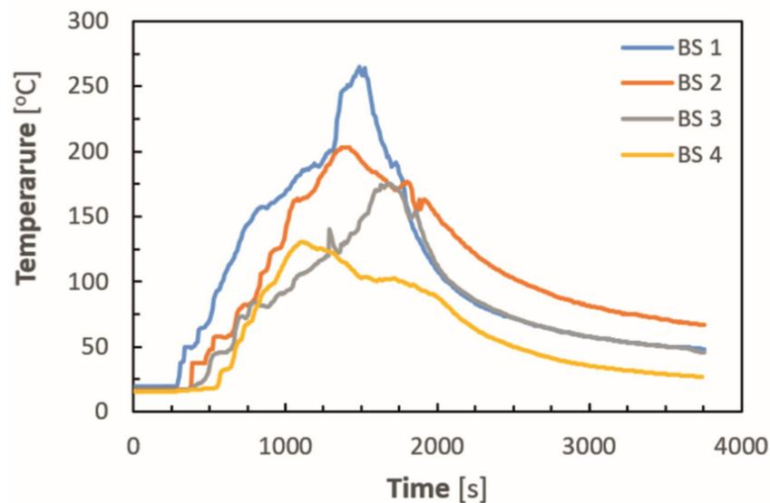
**Figure 6.** Average values of temperatures measured during the test in the insulation layer at level 2 (temperature measurement line L2, located 5 m above the combustion chamber).
