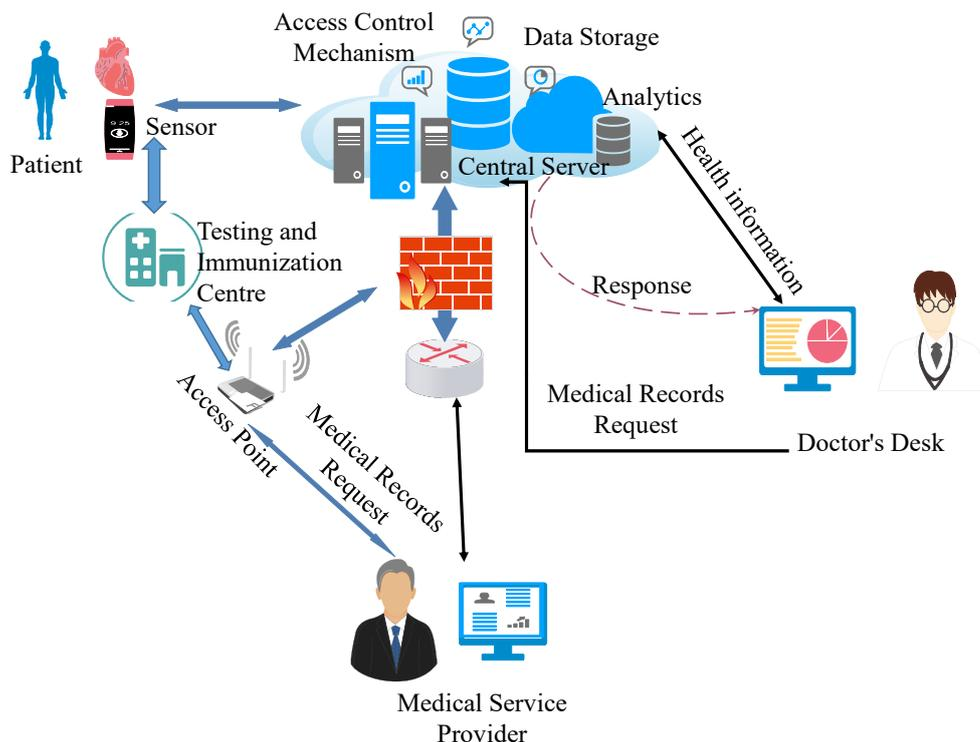
**Figure 1.** Overview of classical cloud-centric EHR management system architecture.
