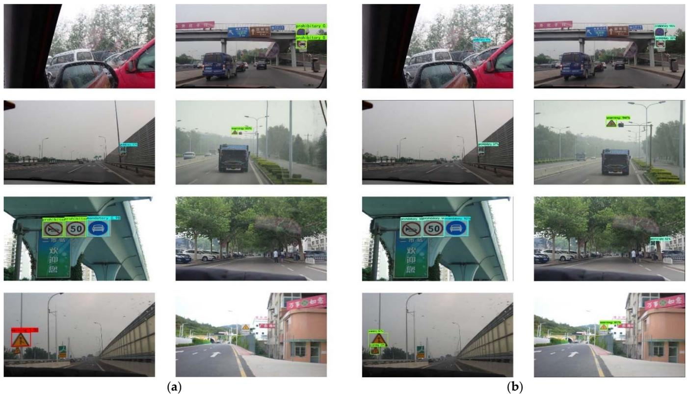
**Figure 8.** Comparison of recognition results of different detection frameworks: (a) YOLOv5; (b) YOLO-FAM.
