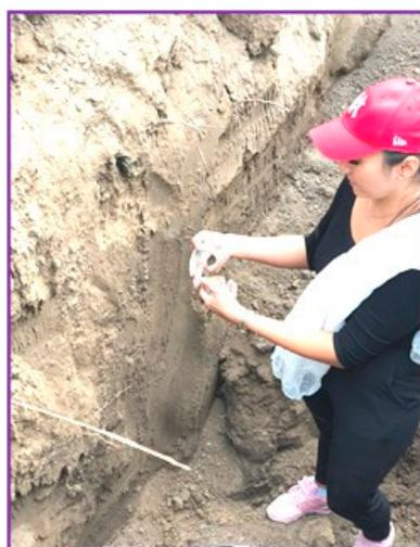
**Figure 8.** A sampling of the soil with undisturbed structure into bins from pit No 2. Photo taken by V. Kulagin and A. Ismagulova.
