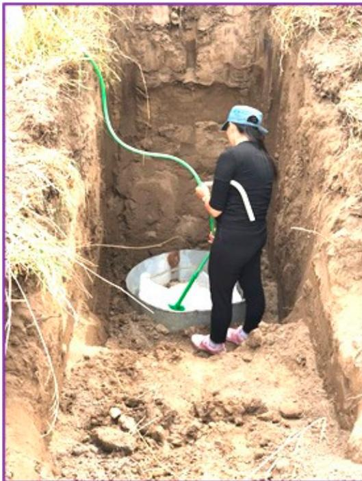
**Figure 10.** A water percolation test in the sand with gravel was carried out at a depth of 2.1 m in the prepared mini pool No. 1 at the Aksu research site. Photo taken by V. Kulagin and A. Ismagulova.
