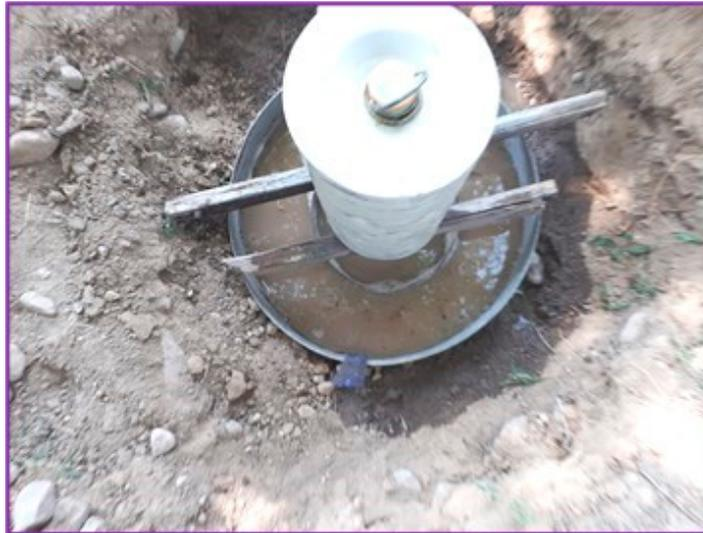
**Figure 9.** A water percolation test in low-permeability loams was carried out in prepared pit No. 1 at the Aksu research site. Photo taken by A. Ismagulova.
