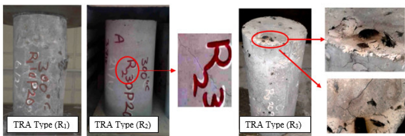
Figure 12. Physical characteristics of rubberized concrete after exposure to 300 °C.
