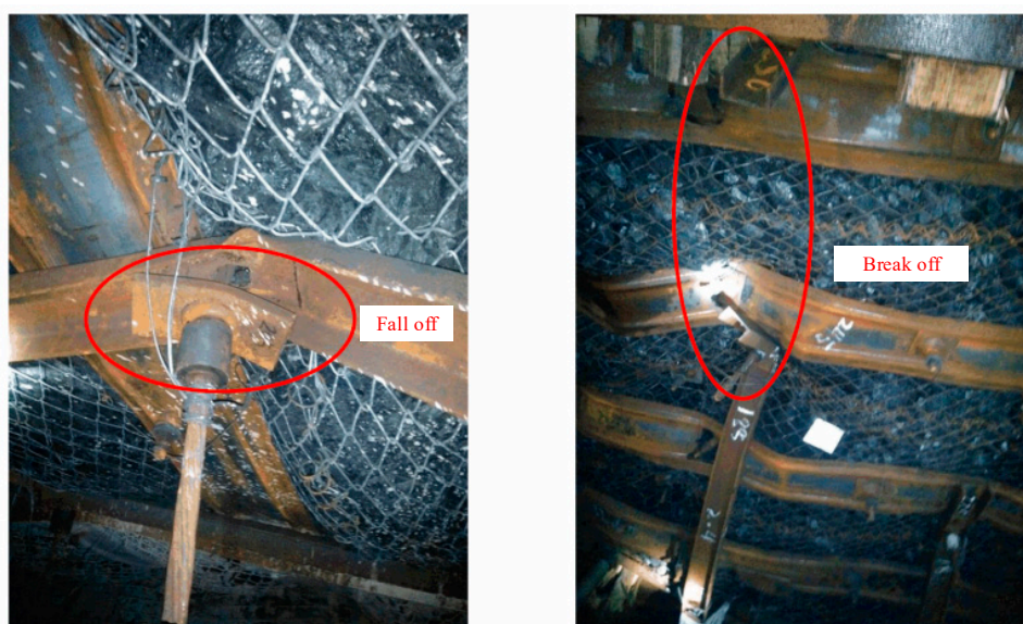
Figure 4. Diagram of field support failure.
