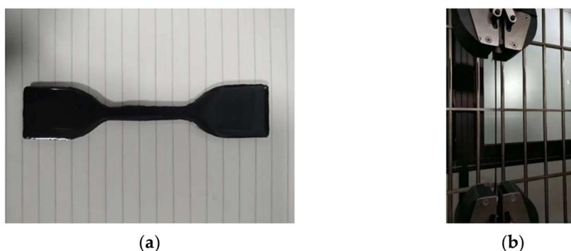
**Figure 2.** Tensile test of (a) specimen and (b) test setup.
