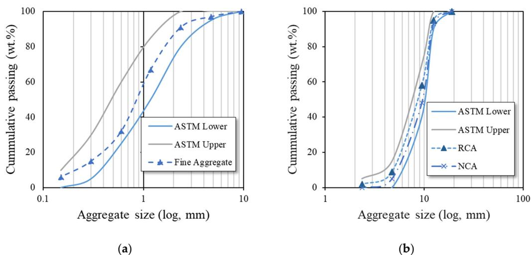
**Figure 4.** Gradation charts: (a) fine aggregate; (b) NCA and RCA.
