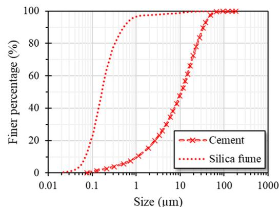
Figure 1. Gradation of cement and SF.
