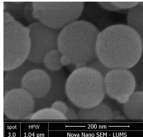
**Figure 3.** SEM image of SF at 200 nm resolution.
