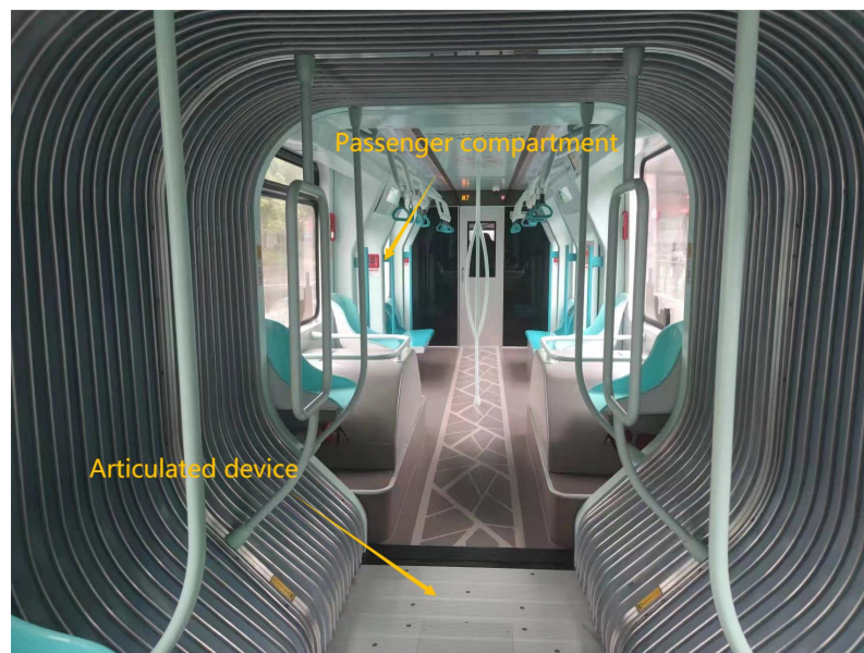
Figure 2. Passenger compartment and articulated device of the multiunit articulated rubber-wheel autonomous rail rapid transit system.
