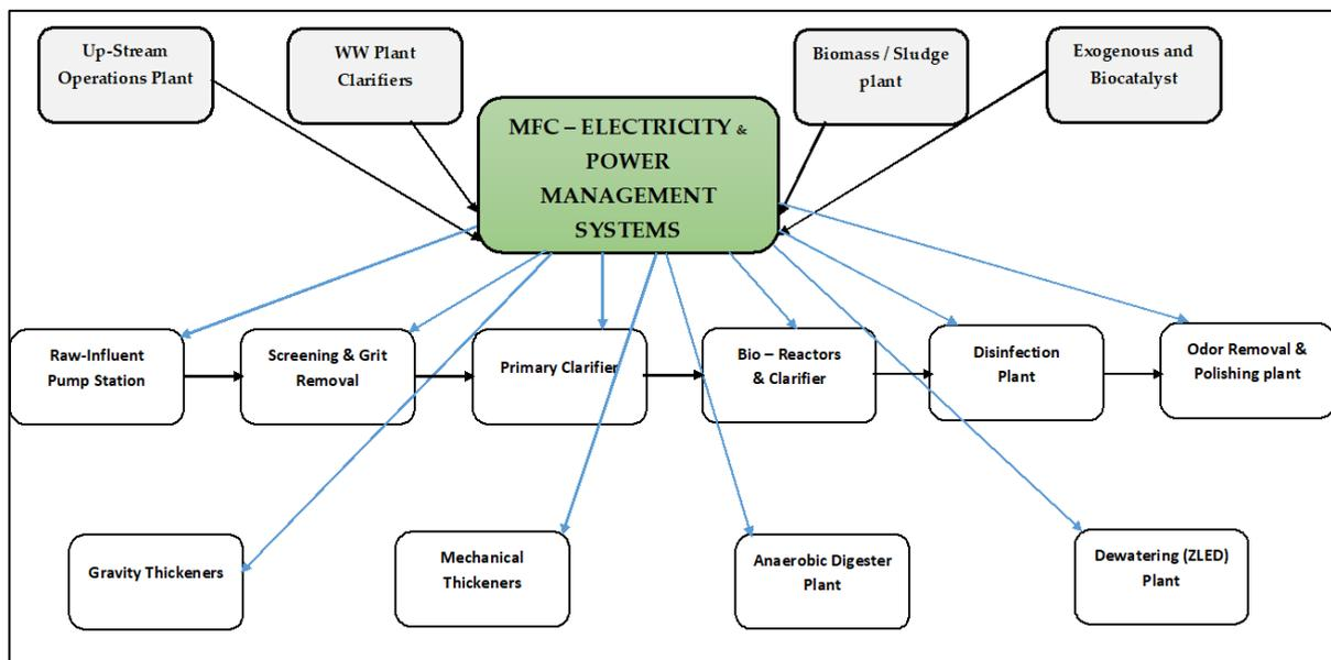
**Figure 6.** Typical waste management hierarchy that incorporates MFC technology as a viable solution for both waste disposal and energy shortages.
