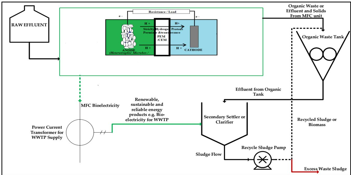
**Figure 4.** Summarized flowchart of the possible practical installation of an MFC at the secondary treatment stage, feeding into a downstream solid contacting vessel, a secondary settler, solids pumps, and a recycled sludge stream to the solids tank.
