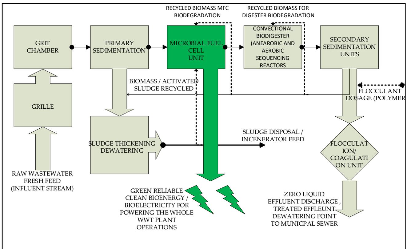
**Figure 5.** Process block diagram for MFC installation in a conventional wastewater treatment plant at the primary sedimentation stage for enhanced substrate concentrations.
