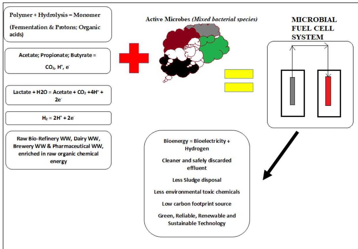
Figure 2. Summary of the wastewater treatment framework in an MFC for bioelectricity production.
