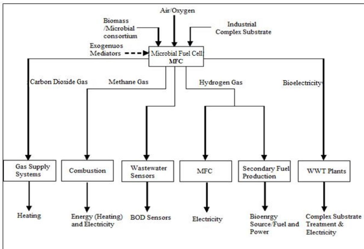
**Figure 3.** Outline process block diagram (PBD) for the practical applications of MFCs.
