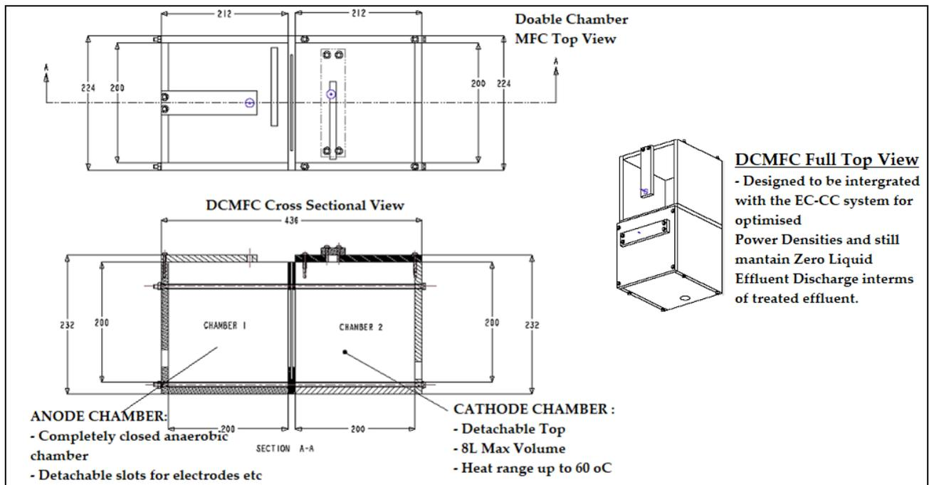
Figure 8. Proposed novel large double-chamber open-top air-cathode MFC (LDCMFC).
