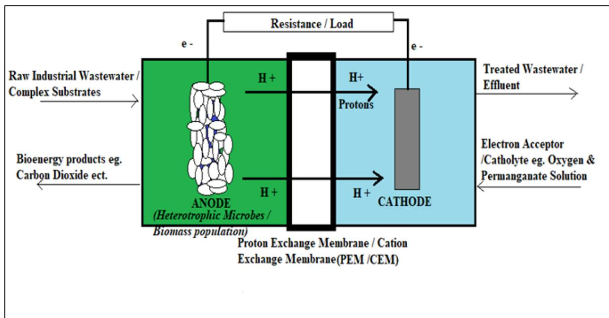
**Figure 1.** Summarizes typical process functioning of an MFC chamber, all compartments outlined.
