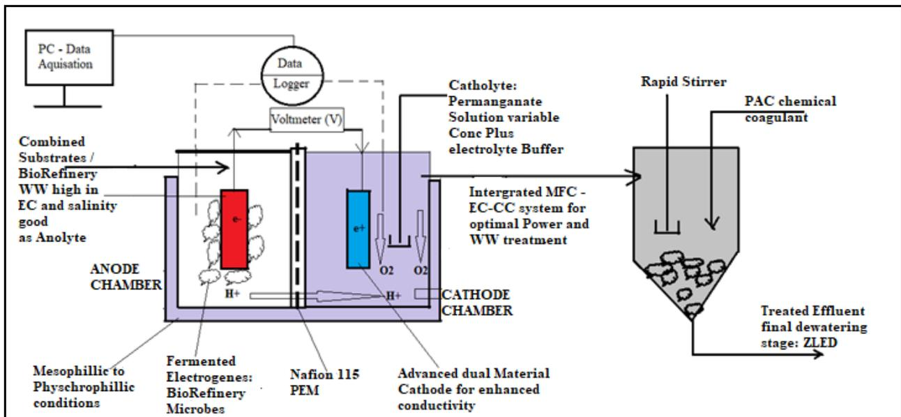
Figure 9. Summary of the proposed integrated lab-scale DCMFC–floculator system for enhanced bioelectricity and WWT.
