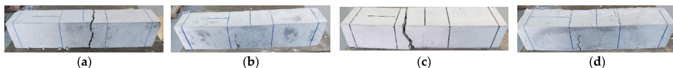
Figure 15. Sample pictures of specimens after the flexural test: (a) N-R60-B-0.0; (b) N-R60-B-1.0; (c) H-R60-B-0.0; (d) H-R60-B-1.0.
