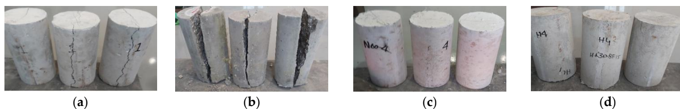
Figure 12. Sample pictures of specimens after the splitting tensile test: (a) N-R60-B-0.0; (b) H-R30-B-0.0; (c) N-R60-B-1.5; (d) H-R30-B-1.5.
