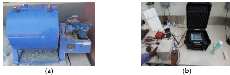
Figure 5. Typical durability tests in progress: (a) Los Angeles abrasion; (b) ultrasonic pulse velocity.
