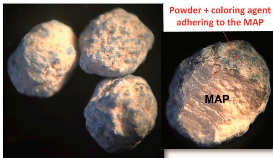
**Figure 3.** Optical microscope images of the MAP + powder (sulfate or carbonate) + adhesive agent + coloring agent. Source: image created by the author Douglas Guelfi.
