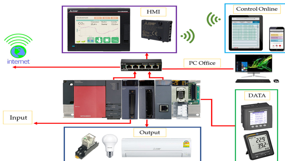
Figure 3. Lighting control system for classrooms.
