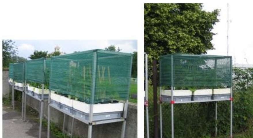
Figure 1. Exposure sites structure of pots with plants placed on Styrofoam and water trays within a special aluminium construction.
