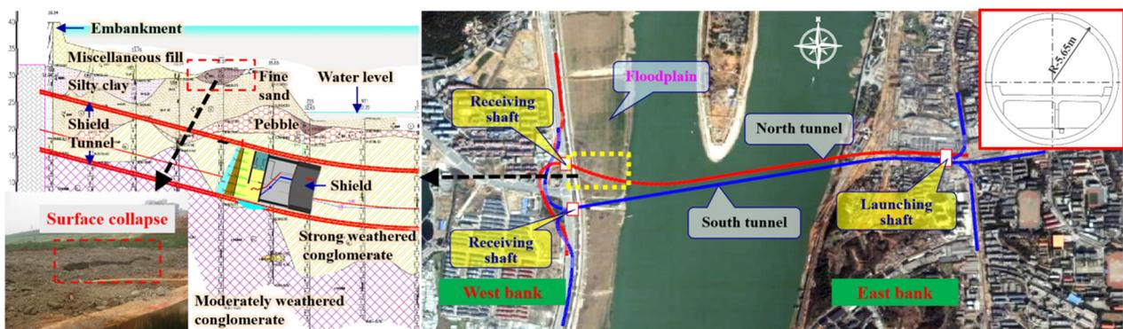
Figure 3. Overview of the underwater tunnels.
