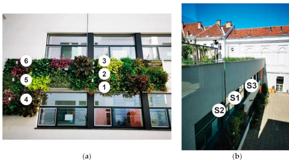
**Figure 7.** Images of the installed sensors at Schuhmeierplatz School: (a) position of the temperature and humidity sensors in front of the living wall; (b) position of the surface temperature sensors above the living wall, and position of the weather station on the roof terrace.
