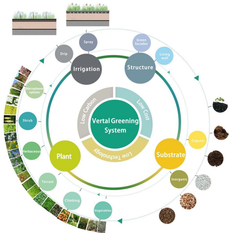
Figure 3. Composition of vertical greening system.
