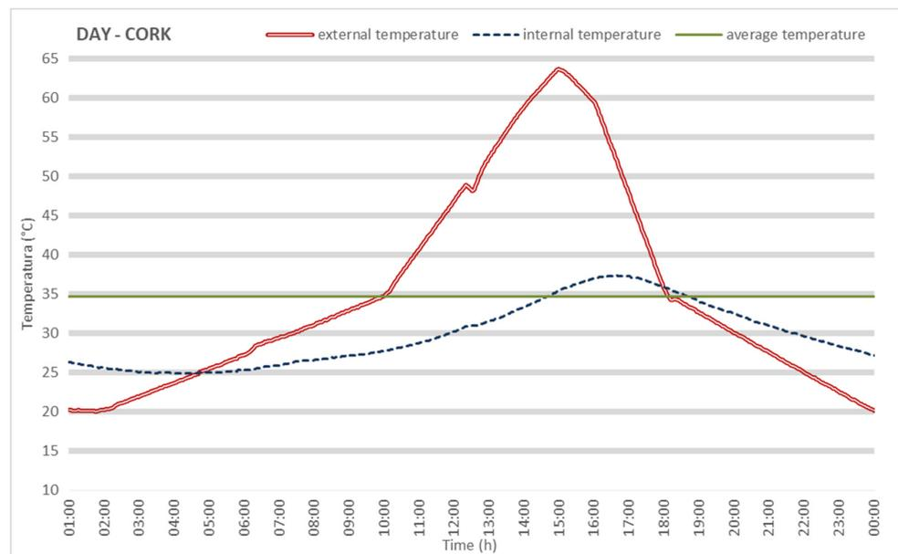
**Figure 8.** Sine waves reproducing the external surface temperature on the ETICS (red line) with ICB as the thermal insulating material, the internal surface temperature on the ETICS (blue line), and the average external temperature (green line) on the hottest day of the year.
