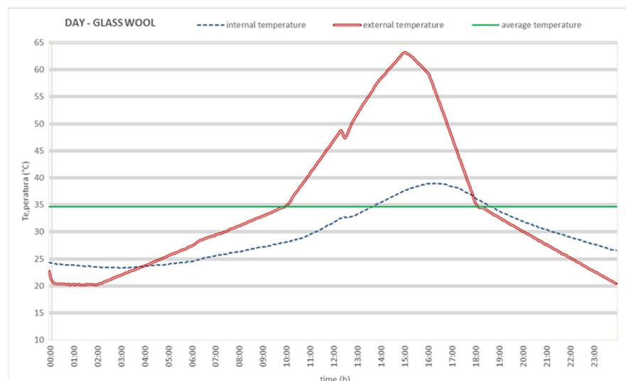
**Figure 7.** Sine waves reproducing: the external surface temperature on the ETICS (red line) with GW as the thermal insulating material, the internal surface temperature on the ETICS (blue line), and the average external temperature (green line) on the hottest day of the year.
