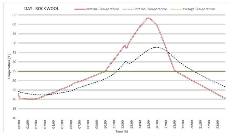
**Figure 6.** Sine waves reproducing the external surface temperature on the ETICS (red line) with MW as thermal insulating material, the internal surface temperature on the ETICS (blue line), and the average external temperature (green line) on the hottest day of the year.
