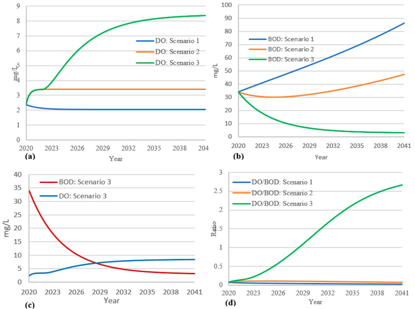
**Figure 8.** Simulation results of three scenarios, (a) DO, (b) BOD, (c) Sustainable water quality and (d) DO/BOD ratio.
