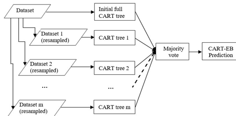
**Figure 4.** Flowchart of the CART-EB algorithm.
