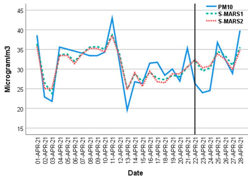
Figure 13. Forecasting of the measured PM<sub>10</sub> levels for the last 28 days using the stacked S-MARS models. The predicted values are plotted to the left of the vertical line, and data forecasts for the 7-day holdout sample are provided to the right.
