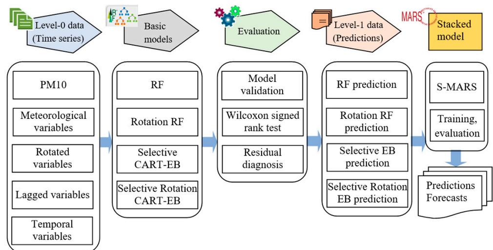
**Figure 3.** Scheme of the proposed stacking framework.
